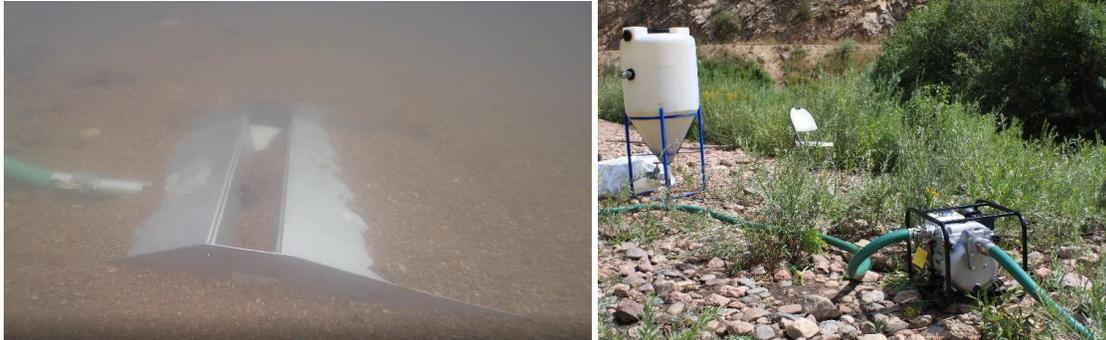
Sand and gravel being deposited into a collector prior to being pumped to shore and volumetrically measured in production time trials
