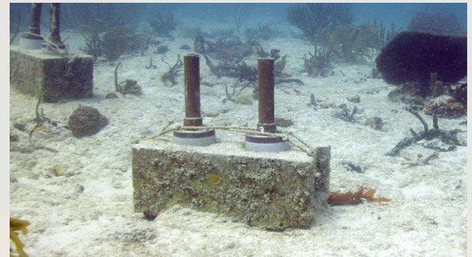
Typical Sedimentation Station
