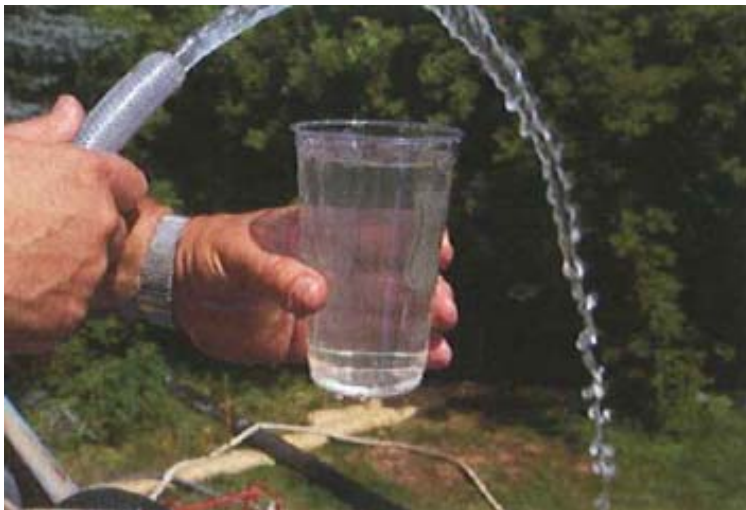
Figure 14. Return lake water after exiting the dewatering system.
