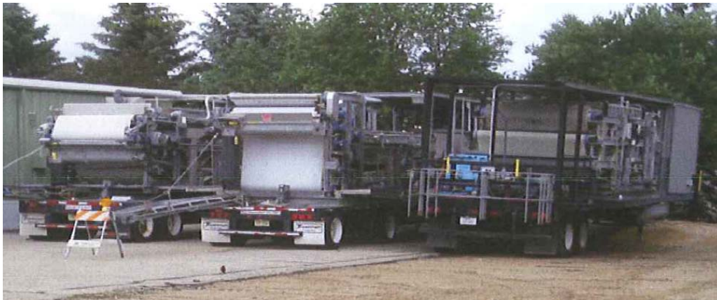
Figure 7. Placement of the portable belt presses.
