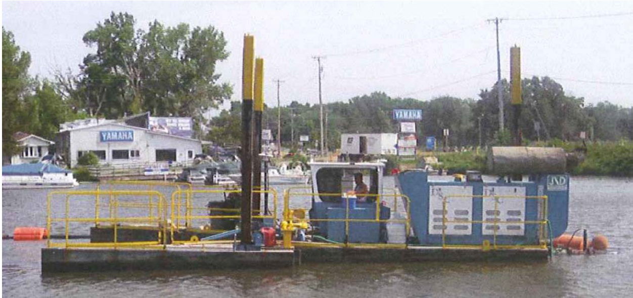
Figure 8. Eight inch DSC Moray swinging ladder dredge positioned in Lake Delavan North Inlet
