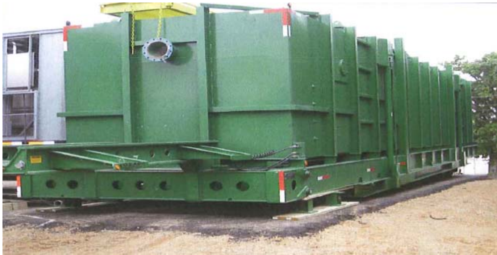
Figure 6. Placement of the portable clarifier tank (in lowered, transport position)
