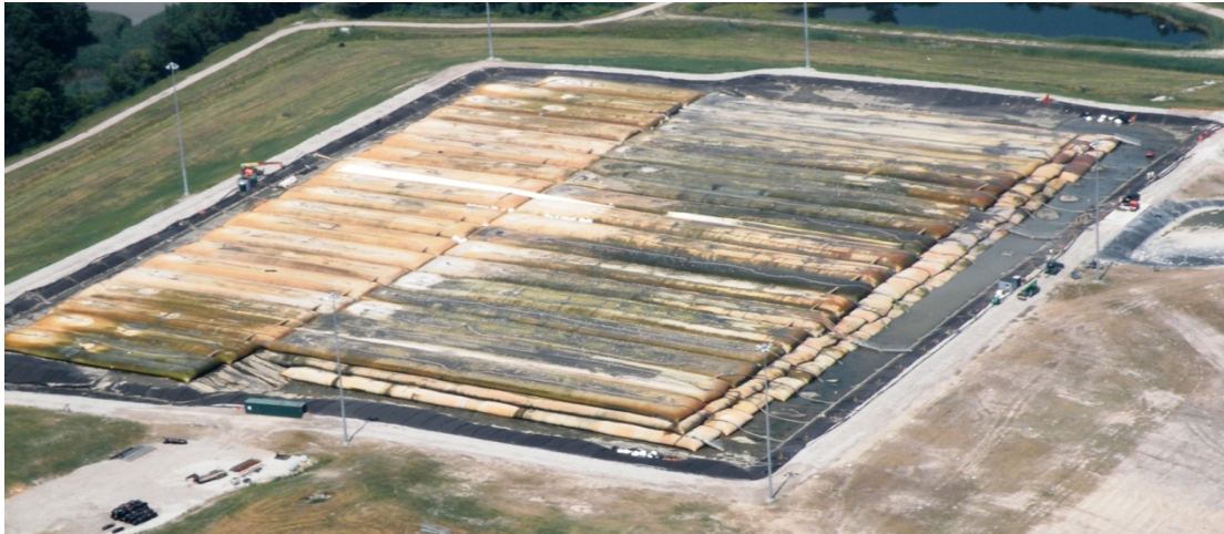
Figure 6. Aerial view of the non-TSCA dewatering pad showing the tiered surface.
