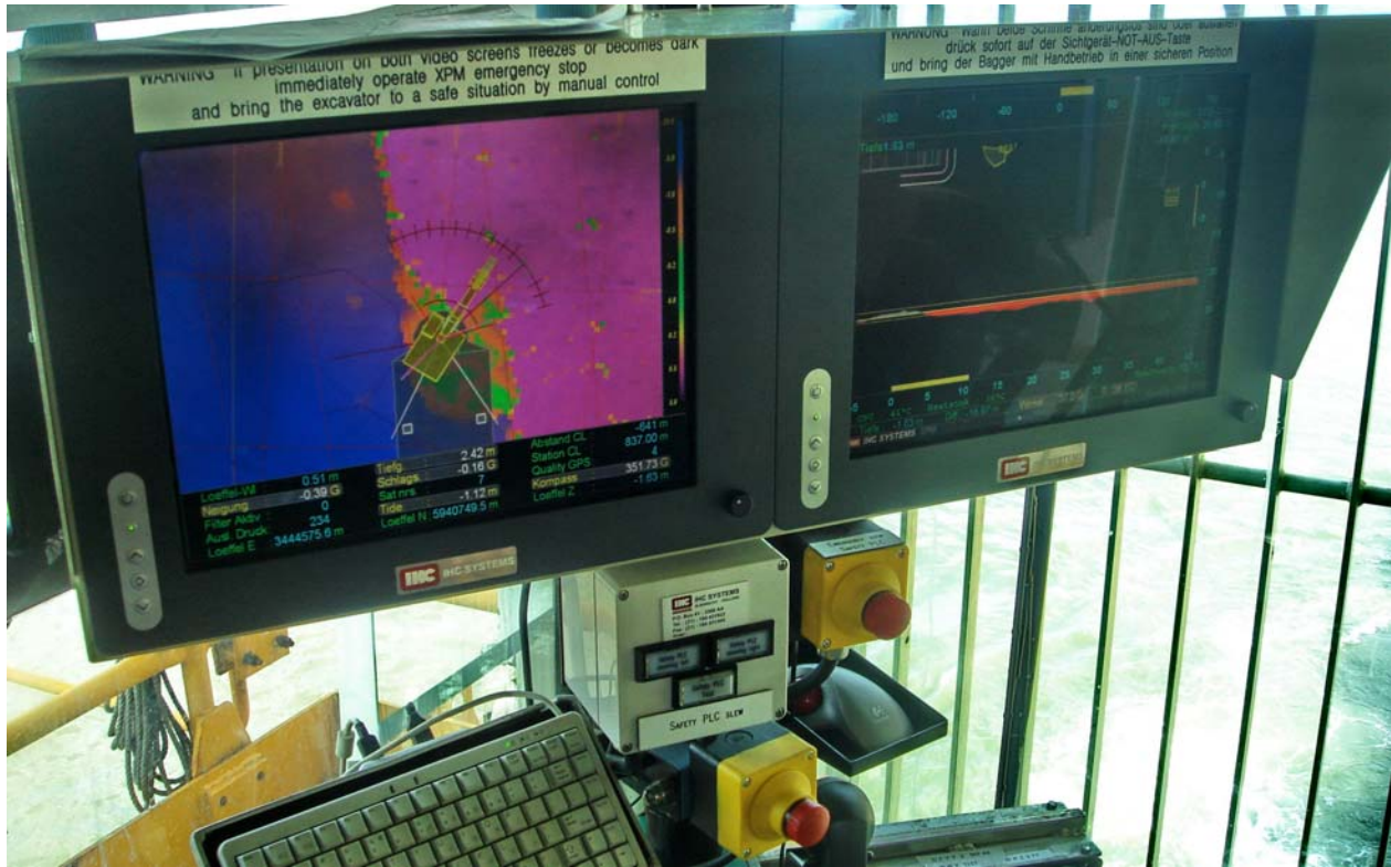
Figure 10. The MP40 pontoon and her nerve centre in the cabin of the Liebherr 995.
