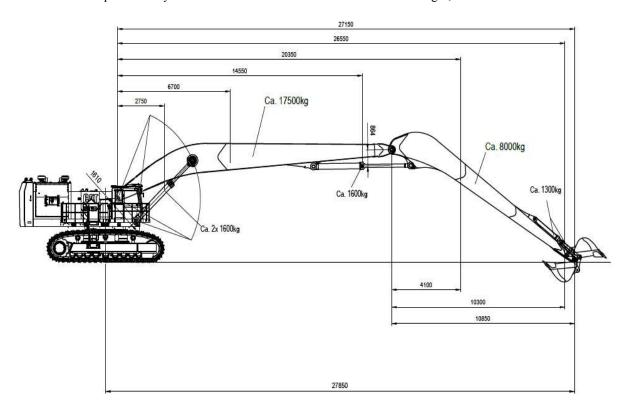
Figure 2. Tipping moment calculation information for customized front design.
