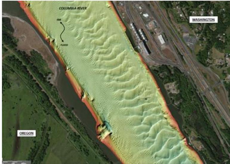
*Lidar image of bathymetry in project area.*
