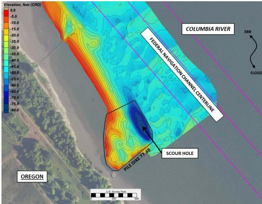
Figure 2A. Pile Dike 77.48 (Oregon flow-lane site) before placement of dredged material.
