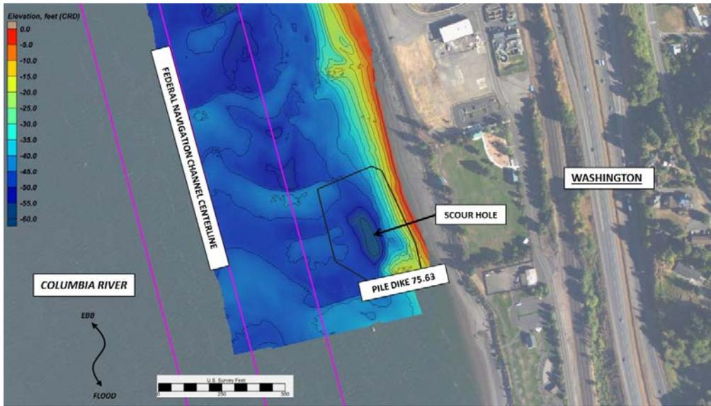
Figure 3A. Pile Dike 75.63 (Washington flow-lane site) before placement of dredged material.
