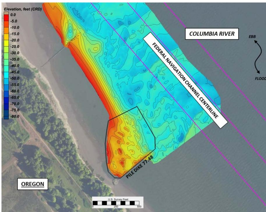
Figure 2B. Pile Dike 77.48 (Oregon flow-lane site) after placement of dredged material.
