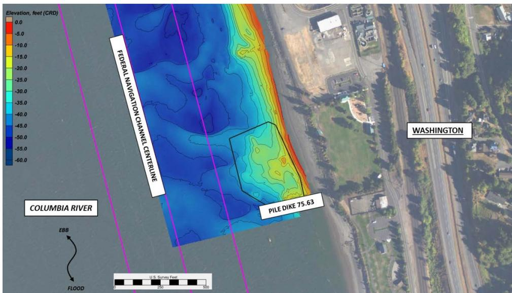
Figure 3B. Pile Dike 75.63 (Washington flow-lane site) after placement of dredged material.
