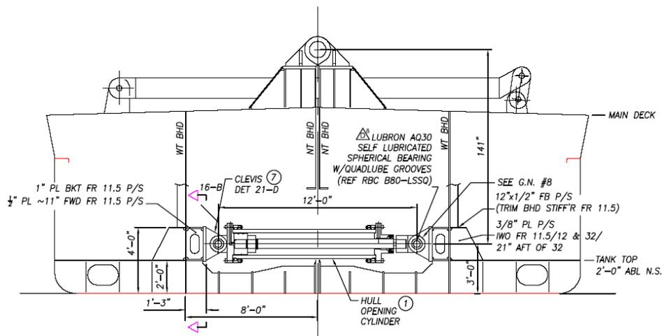
**Hopper Cylinder Retracted, Hopper Closed**
