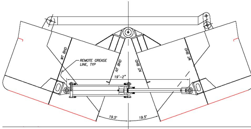
**Hopper Cylinder Extended, Hopper Open**
