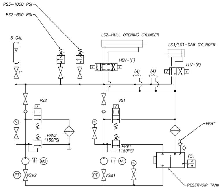
**Simplified Hopper Hydraulic Schematic**
