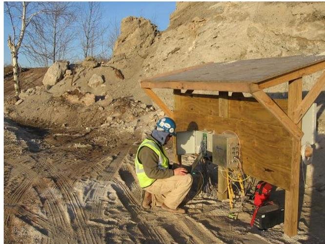
**Figure 9. The CQA/environmental monitoring engineer monitors geotechnical instruments installed by the RAC weekly, with data submitted for analysis by engineers from both organizations.**
