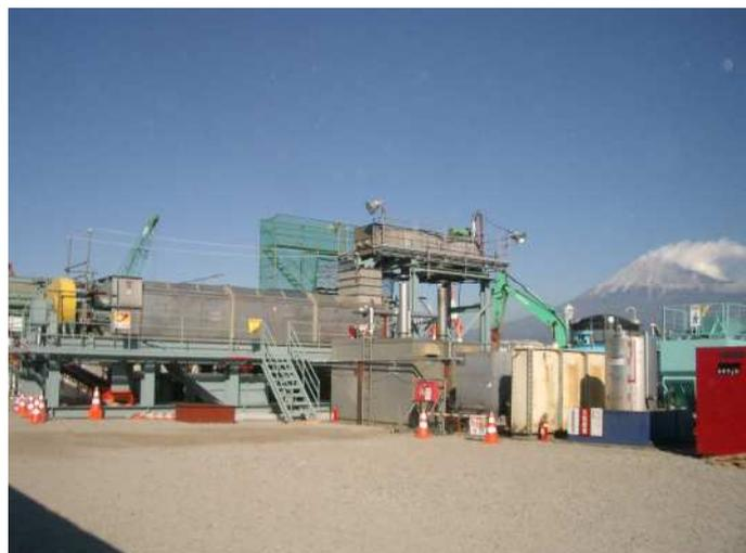
Photograph 2. Dewatering system (one screw press of 1,350-mm diameter).
