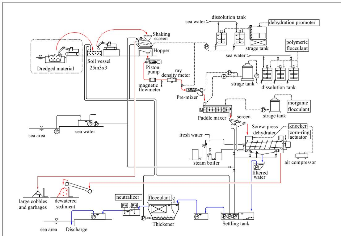
Figure 6. Flow of operation steps.
