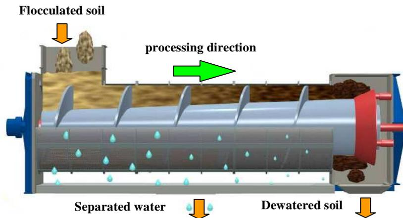
Figure 1. The principles of Eco-screw.
