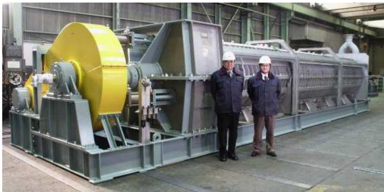
Photograph 1. Screw press of 1,350-mm diameter.
