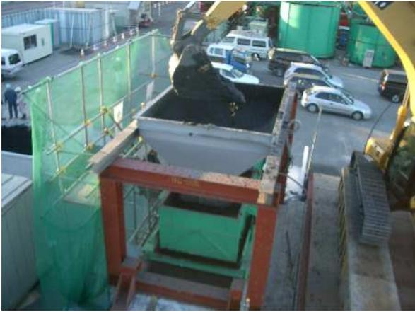
**Photograph 6. Inputting the sediment.**
