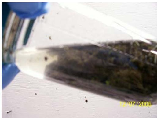
**Figure 9. Dewatering biosolids in a 250-mL sample jar after addition of Solve 213J (300 ppm).**
