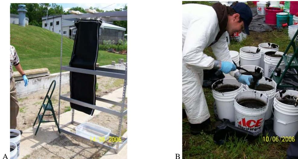
**Figure 1. A) Geotube® hanging bag dewatering performance trial. B) Sediments were collected for analytical testing (e.g., contaminants, percent dry weight solids).**
