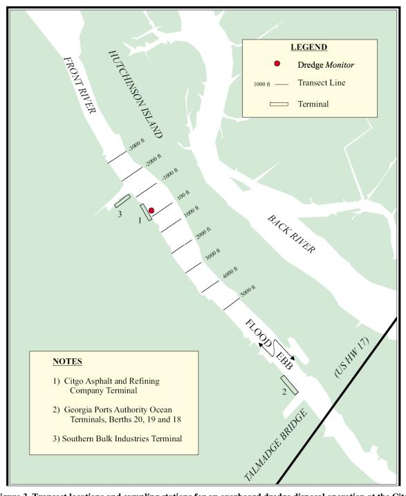
Figure 3. Transect locations and sampling stations for an overboard dredge disposal operation at the Citgo Terminal.
