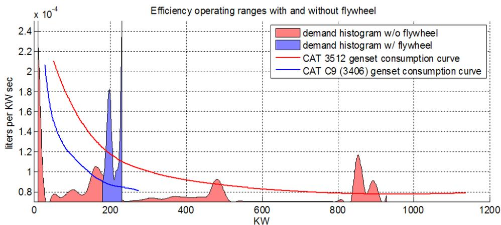
**Figure 10. Power demand histograms and efficiency curves.**
