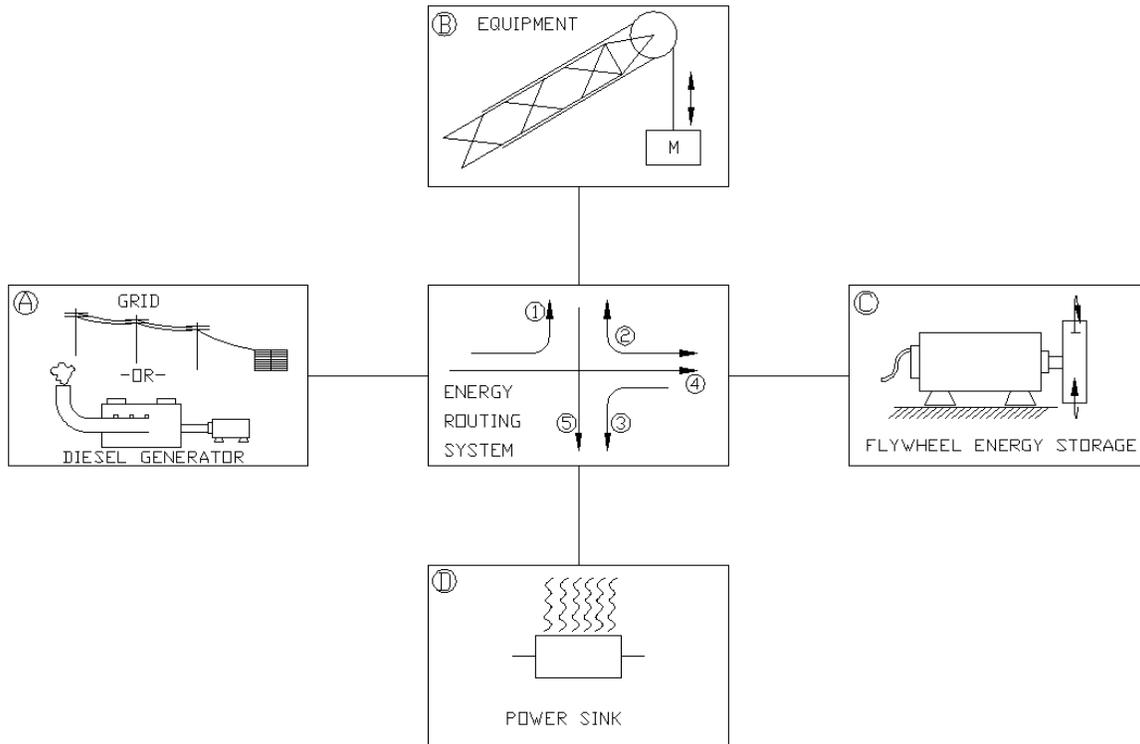
**Figure 3. Power routing topology.**
