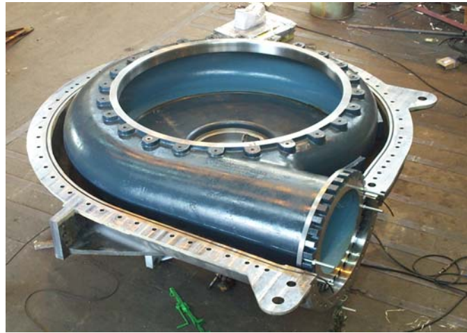
Figure 5. Double wall dredge pump during assembling of inner casing.
