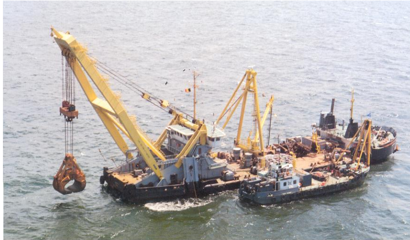
Fig. 3 'Norma' as floating shearlegs
