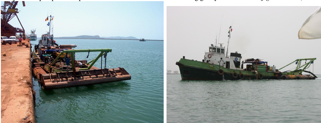
Fig. 10 and fig. 11 Tug 'Geer' as bed leveller
