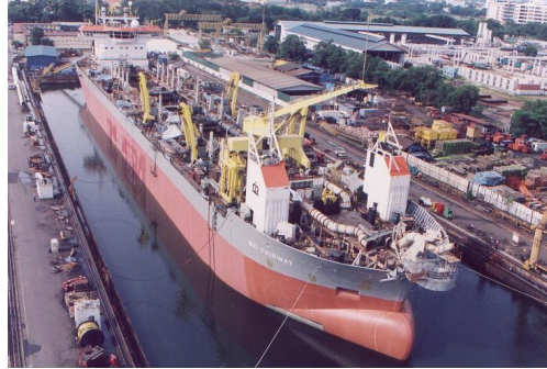
Fig. 37 'WD Fairway' in refloating condition
