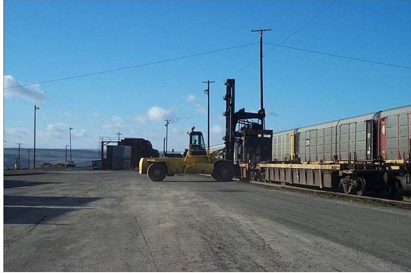
Figure 11. Top-pick lifting 6.1 m (20.0 ft.) shipping container from a rail car.
