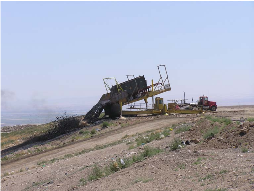
Figure 14. Self-tipper tipping a container of dredge material.
