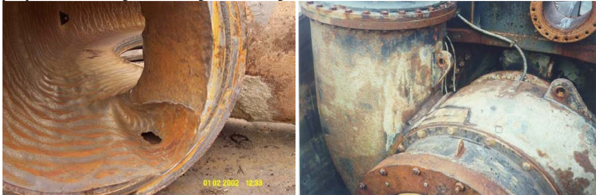
Figure 16. Local wear for too high and too low flow
