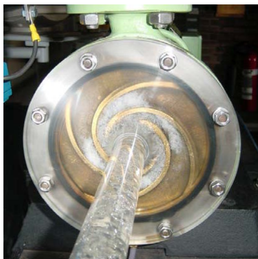
Figure 10. Boiling water “cavitation” in an impeller
