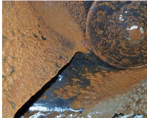
Figure 11. Impeller with cavitation erosion
