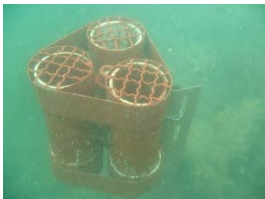
Photo 6. Three sedimentation traps are fixed at each site located on the reef slope close to the coral LIT sites. The height of the trap from the reef surface to the opening is 35cm. The sediment traps are held vertically by angle-bars hammered deep into the ground in an area of dead coral. The actual dimension of the sediment trap is: height 15cm and Ø 5cm.
