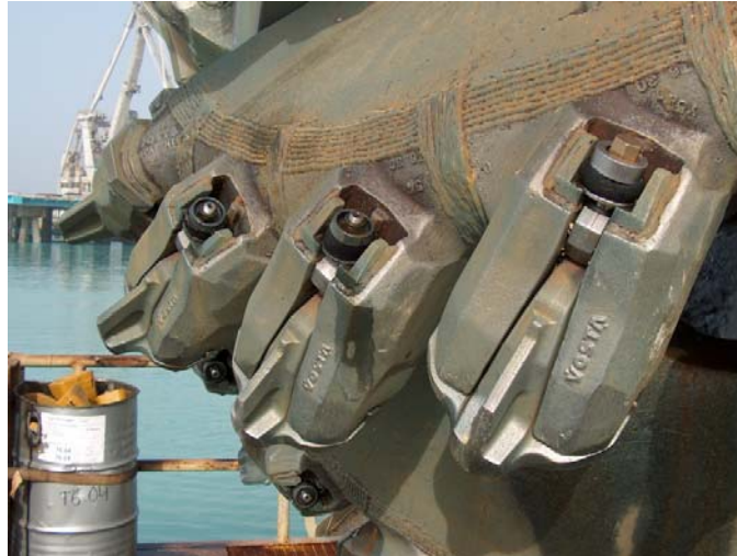
Figure 11. No visible wear after working in hard rock
