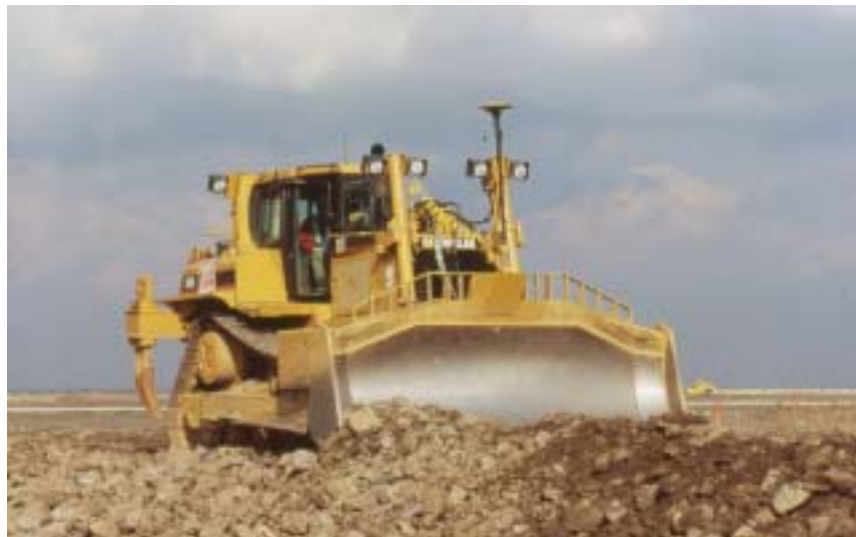
Figure 11. Bulldozer equipped with GPS.
