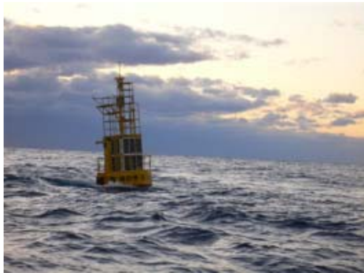
Figure 17. Experimental GPS wave measuring buoy.
