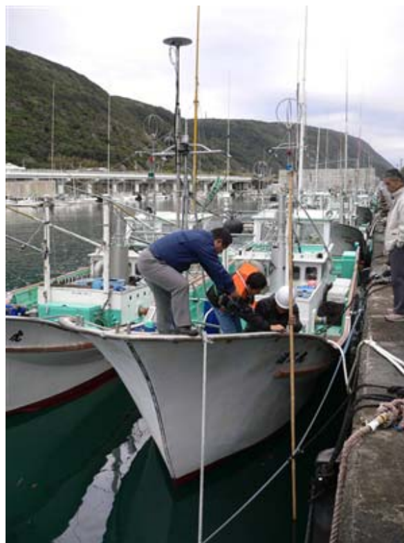
Figure 19. Small boat equipped with RTK-GPS.
