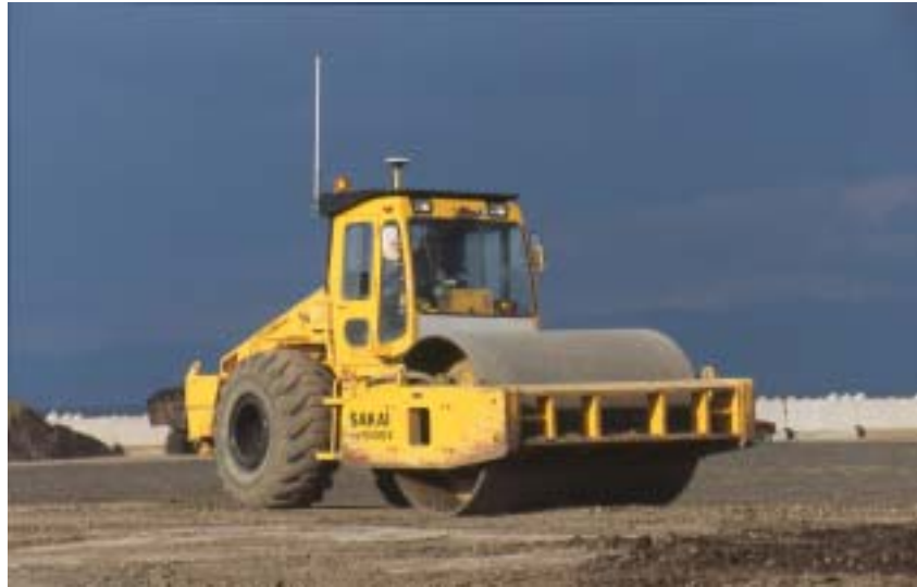
Figure 12. Vibrating roller equipped with GPS.
