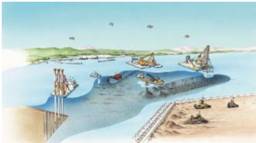
Figure 2. General view of utilizations of GPS in various maritime construction work.
