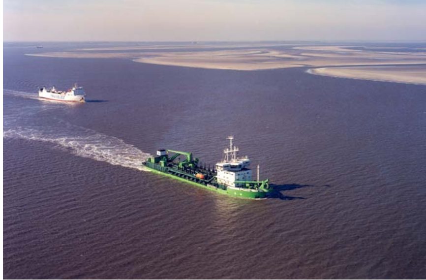
Figure 3. Suction hopper dredger at work in the Scheldt estuary.
