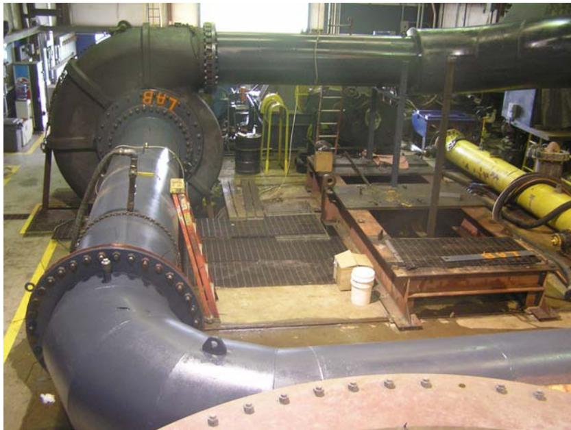
Figure 9. LHD-38x38-58(60.4) C/4HE pump on GIW test stand.
