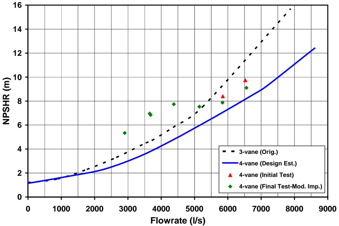
Figure 14. Test data comparison to design estimate for flow-rate versus NPSHR at 307 rpm operation.
