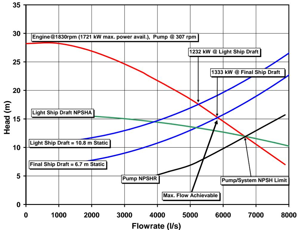
Figure 1. Existing 3-vane LHD58 pump @ 307 rpm filling hopper with water at an average flow-rate of 5600 l/s (88,772 gal/min).
