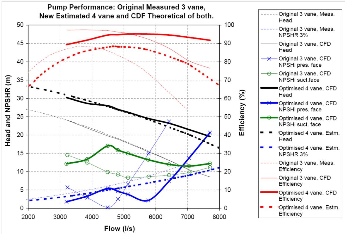
Figure 6. Summary of CFD analyses for the original and final designs at 307 rpm.
