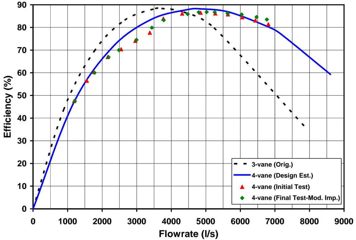
Figure 13. Test data comparison to design estimate for flow-rate versus efficiency at 307 rpm operation.
