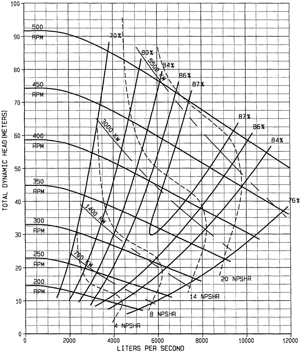
Figure 15. New 38x38LHD58(60.4) multi-speed water performance curve based upon test data.
