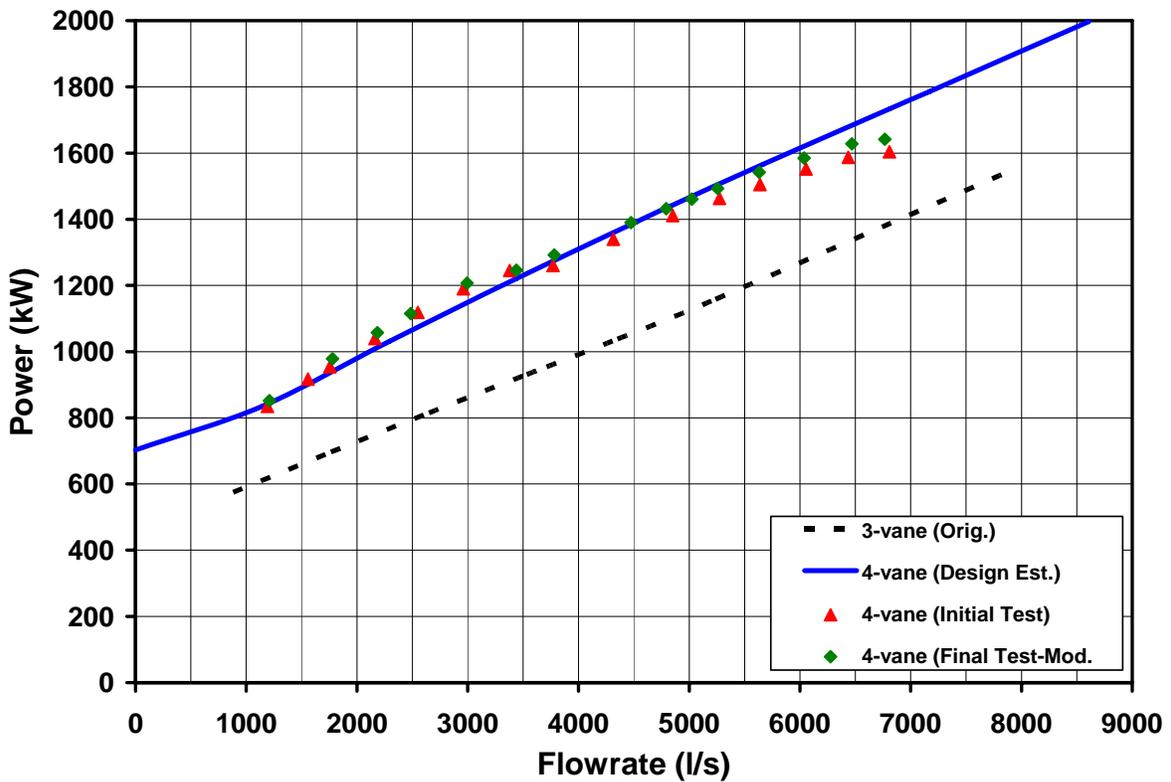
Figure 12. Test data comparison to design estimate for flow-rate versus power at 307 rpm operation.
