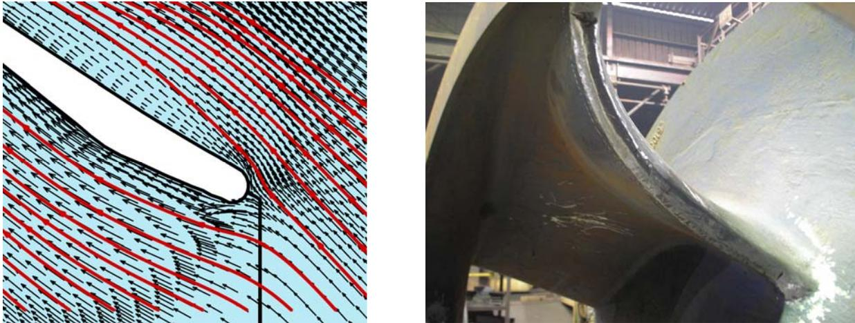
**Figure 3. Optimization of the inlet edge angle resulting in twisted vane inlet geometry.**
