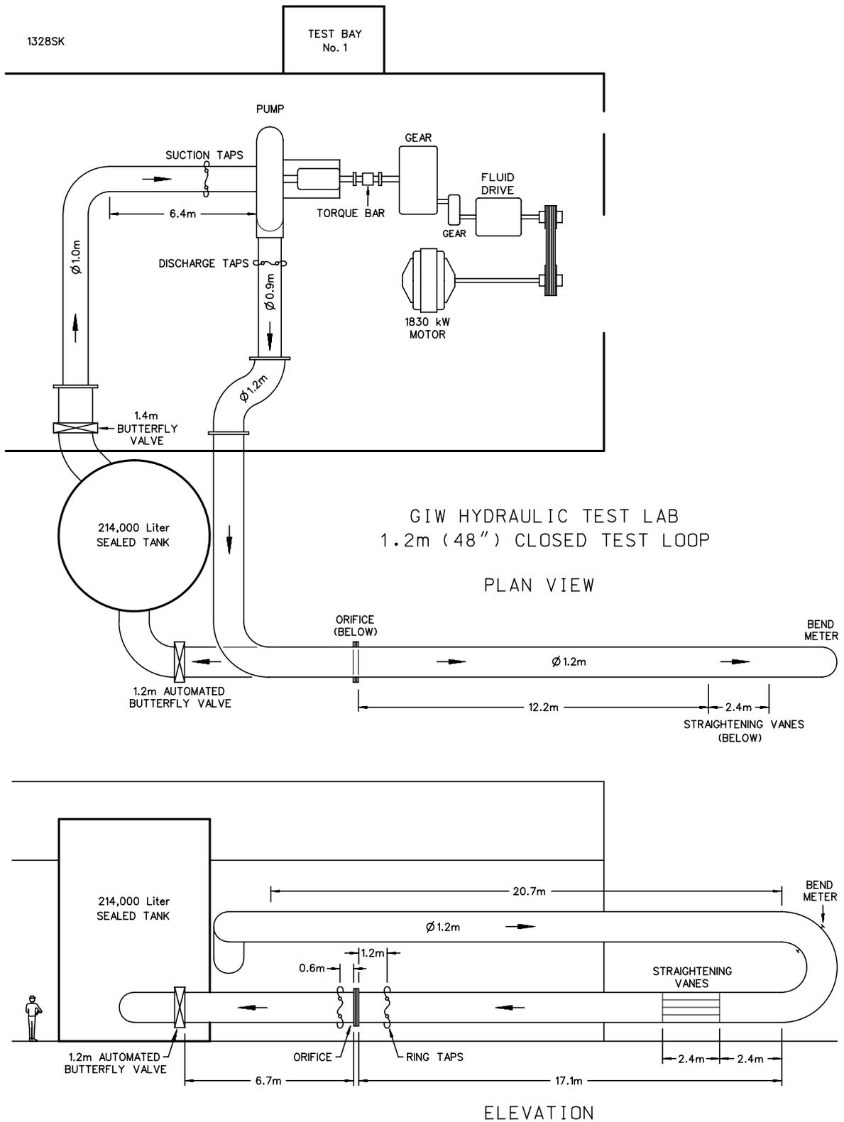
Figure 10. GIW 1.2 m (48 inch) diameter closed loop test system.
