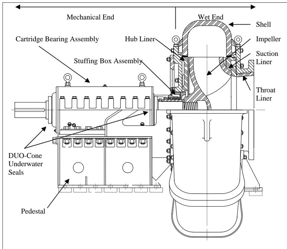
**Figure 8. Bare-shaft LHD-38x38-58(60.4) pump assembly.**
