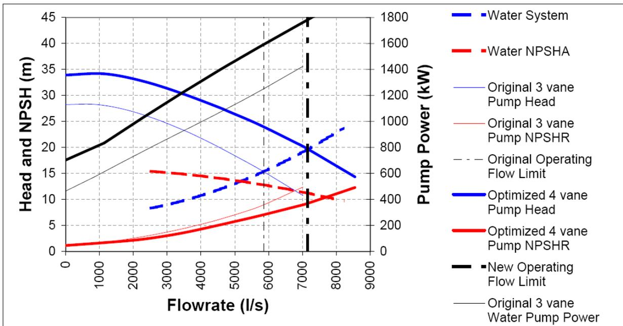
Figure 7. Estimated maximum operating condition for optimized 4 vane design at 307 rpm.
