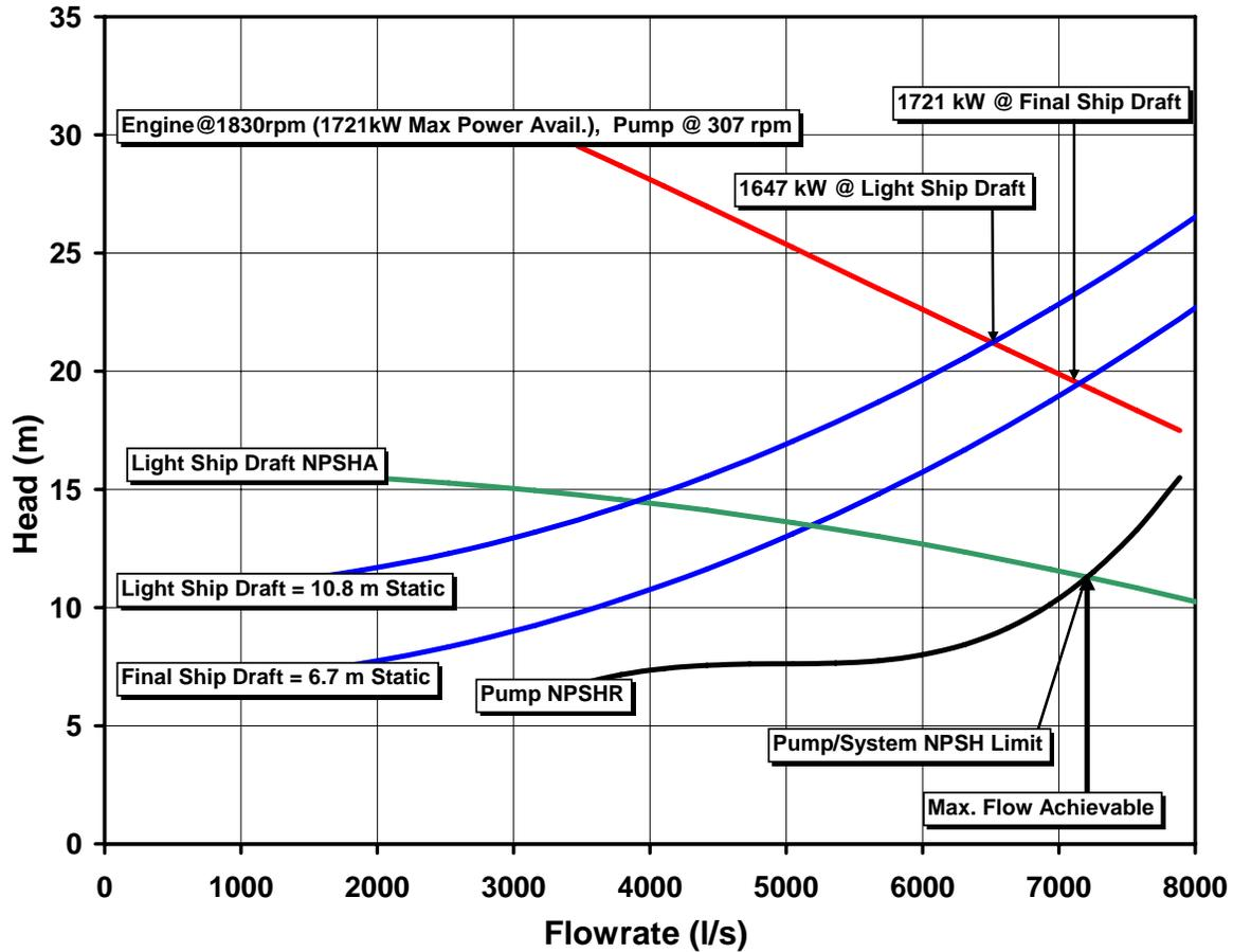
Figure 17. New LHD-38x38-58(60.4) C/4HE pump @ 307 rpm filling hopper with water at an average flow-rate of 6800 l/s (107,794 gal/min).
