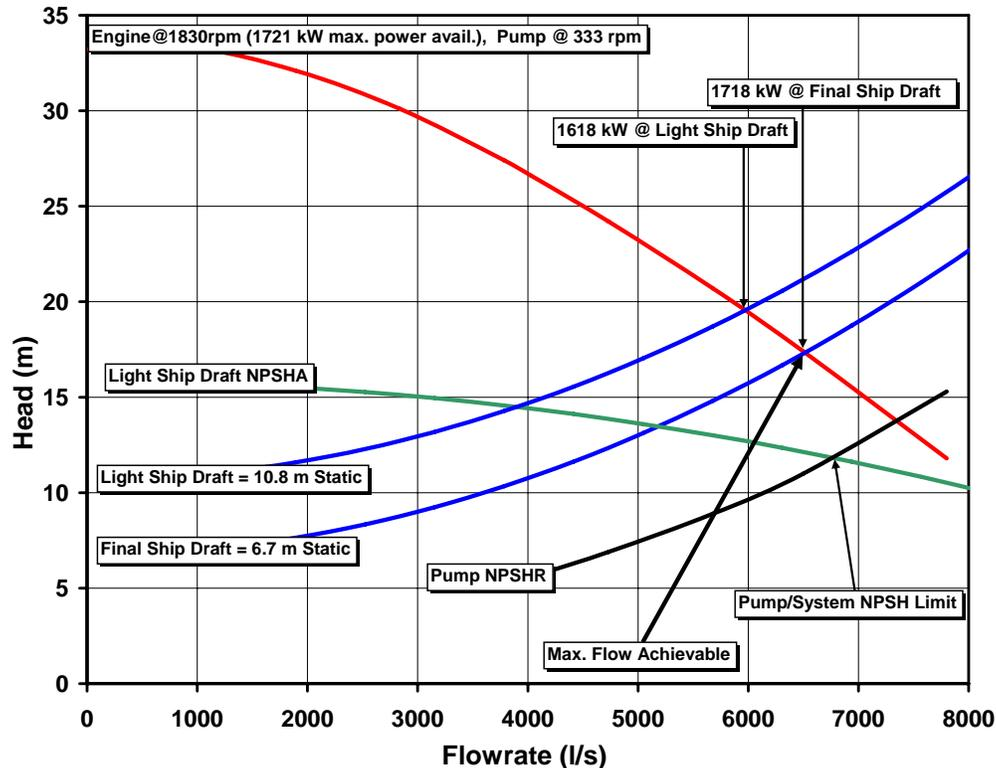
Figure 2. Existing 3-vane LHD58 pump @ 333 rpm filling hopper with water at an average flow-rate of 6225 l/s (98,680 gal/min).
