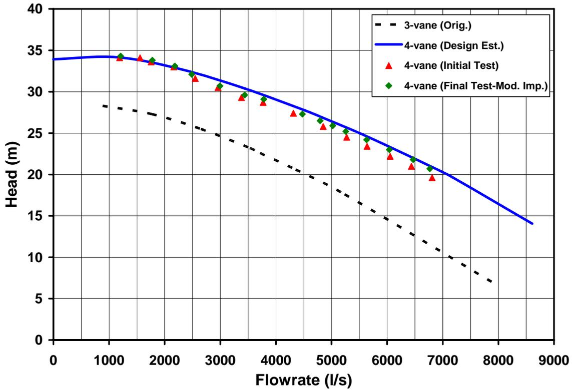
Figure 11. Test data comparison to design estimate for flow-rate versus head at 307 rpm operation.
