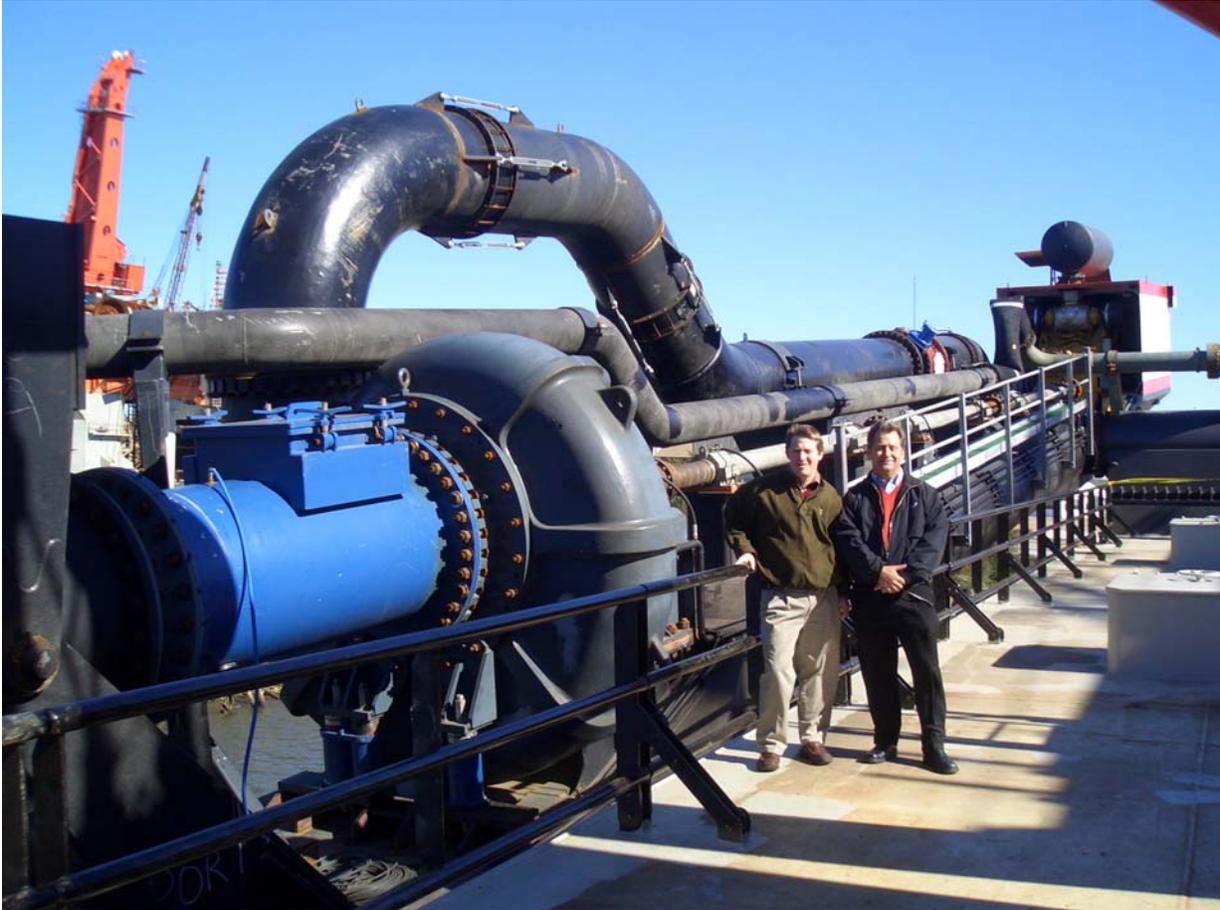
**Figure 16. New 38x38LHD58(60.4) C/4HE pump installed onto one of the *Glenn Edwards* drag arms**
