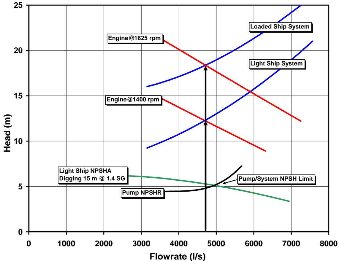
Figure 18. Illustration of hopper solids loading at 1.4 slurry SG and 4750 l/s for 15 m dredging depth on sand.
