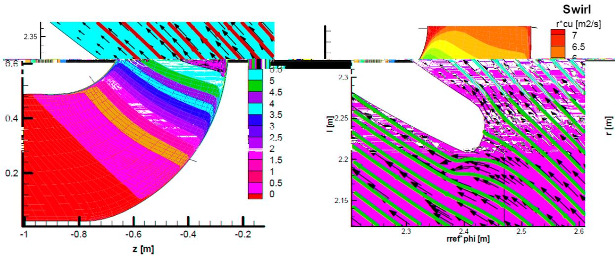
Figure 5. CFD results of optimized 4 vane design.
