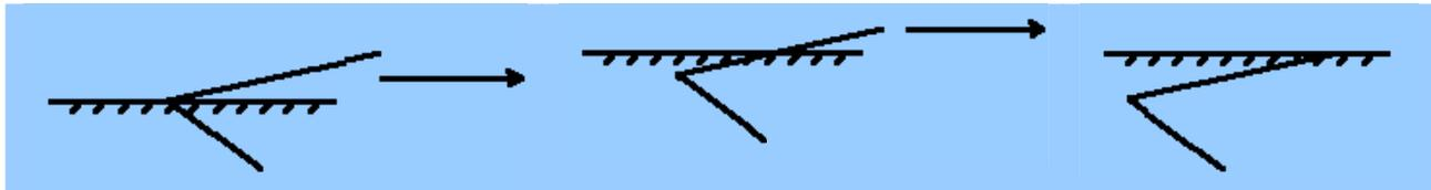
Figure 26. The shank penetrating the soil in phase 3.
