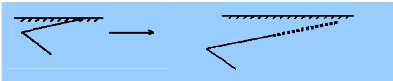
Figure 32. The mooring line penetrating the soil in phase 4.
