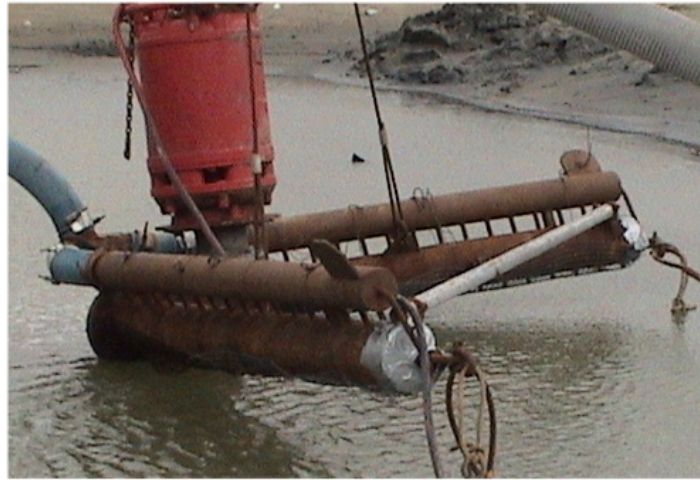
Fig-10 Experimental sand collection device (V type) in beach sand collection.
