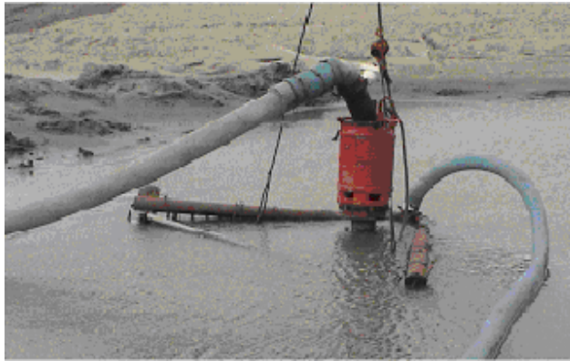
Fig-15 View of beach sand collection device.
