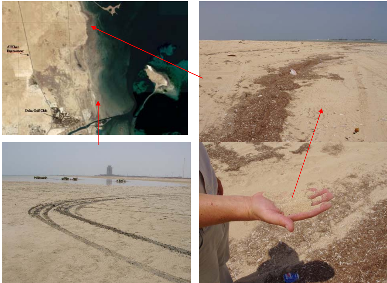
Figure 1. Example of correlation between type of beach and wave exposure. Upper left: location map, North Beach in Doha, Qatar. Note that the southern part is protected by an island and associated reefs and has a muddy tidal flat (photo lower left) whereas the northern part is exposed and has a sandy beach (photos to the right).
