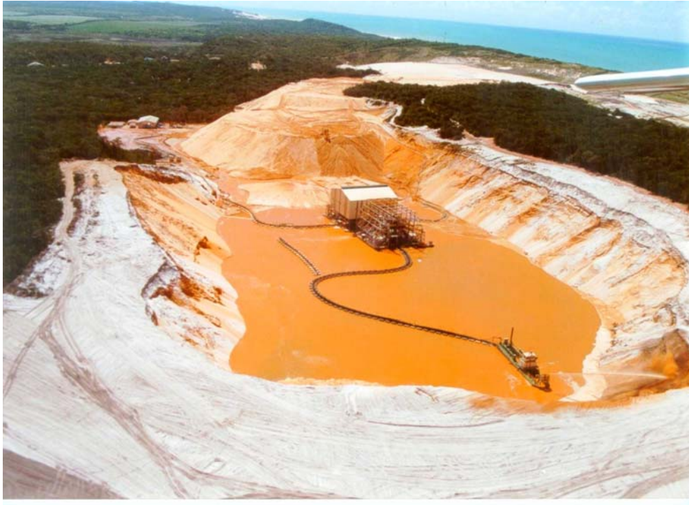
Figure 9. Wheel dredger in pond connected to the floating primary concentration plant.
