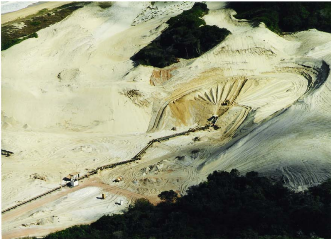
Figure 2. Aerial picture of the dry mining operation showing the funnel shaped trajectory and conveying system to the process plant.
