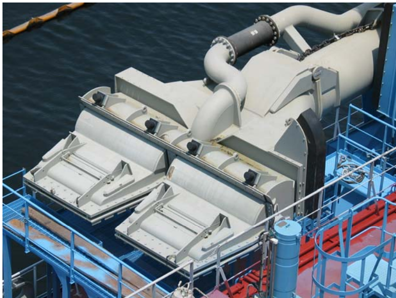
Figure 23. Drag head with turbulence visor of TSHD “Mecca”.
