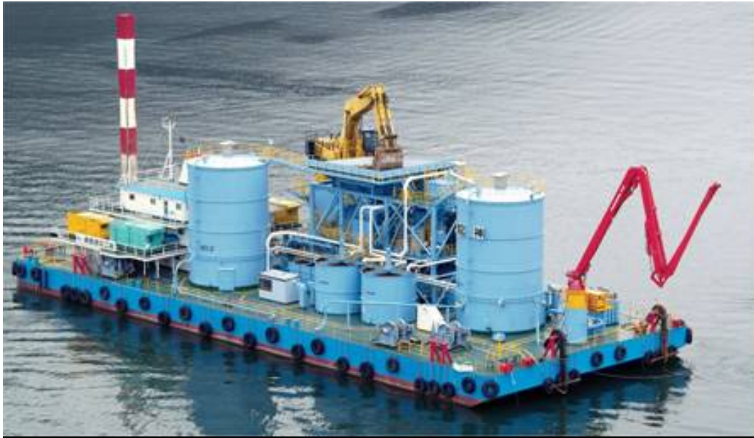
Photo 4. Ryu Jin, lightweight mixing-treatment vessel.
