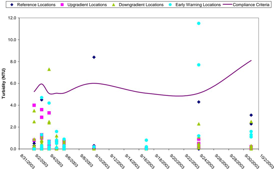
**Figure 3 Turbidity Versus Time During Dredging**
