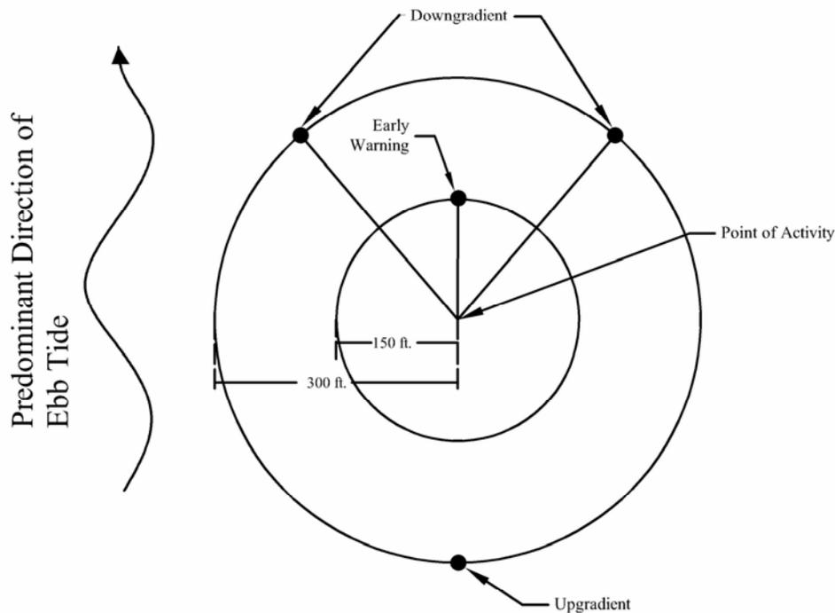
**Figure 2 Compliance Water Quality Monitoring Locations During Dredging**
