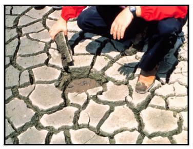
Figure 5. Desiccation Cracks in Fine-Grain Dredged Material
