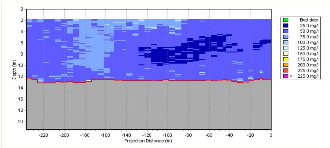
**Figure 15. Vertical profile of TSS on Transect 8 during a flooding tide survey (ODFC).**
