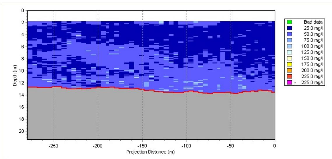
**Figure 6. Vertical profile of TSS on Transect 3 during an ebbing tide survey (ODEC).**
