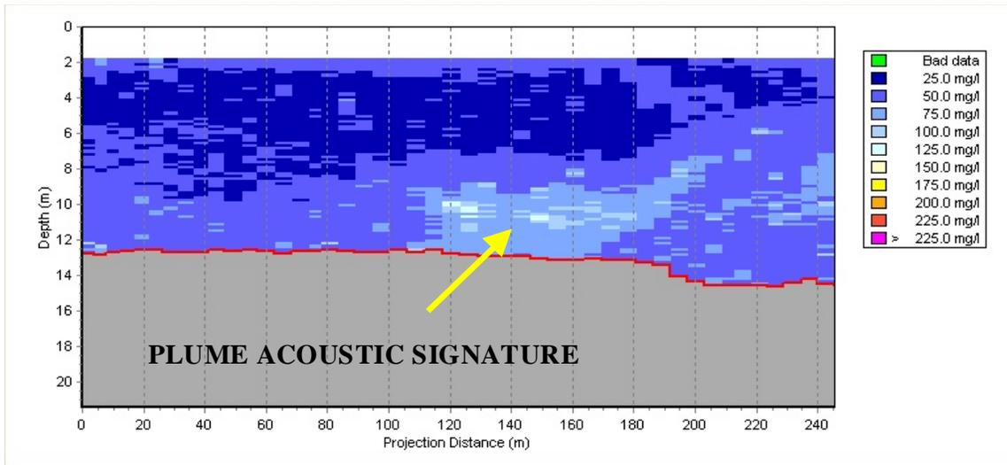
Figure 7. Vertical profile of TSS on Transect 4 during an ebbing tide survey (ODEC).
