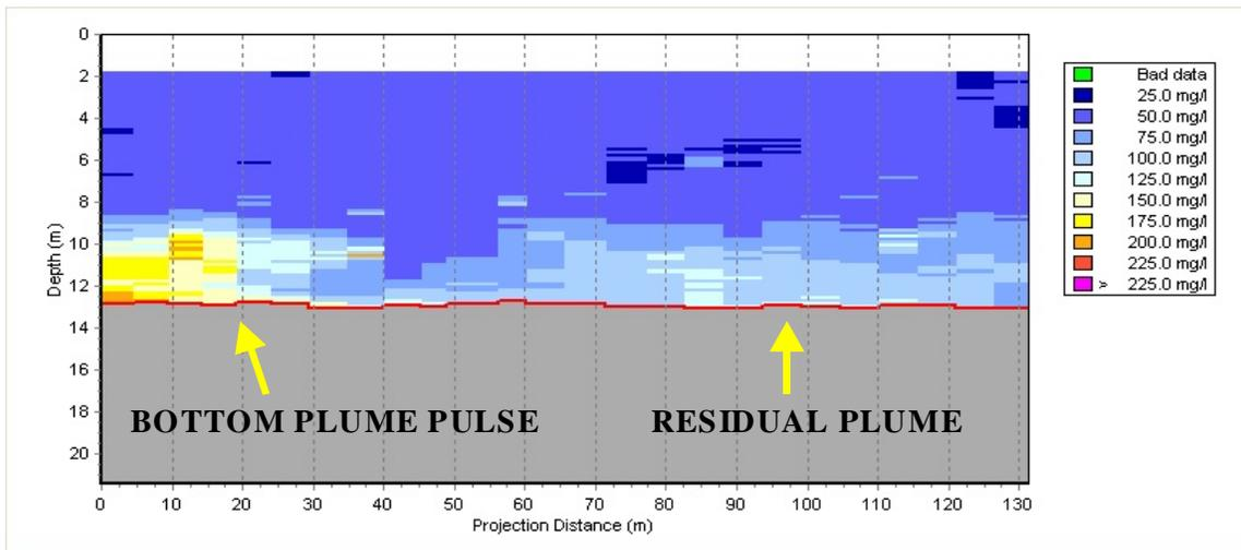
Figure 9. Vertical profile of TSS on Transect 8 during an ebbing tide survey (ODEC).
