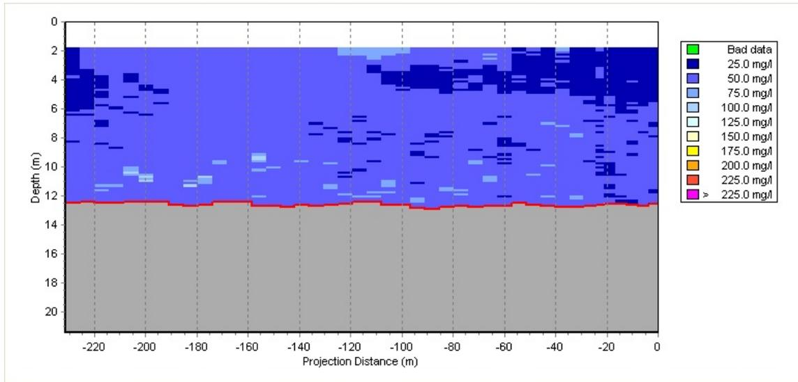
**Figure 16. Vertical profile of TSS on Transect 10 during a flooding tide survey (ODFC).**
