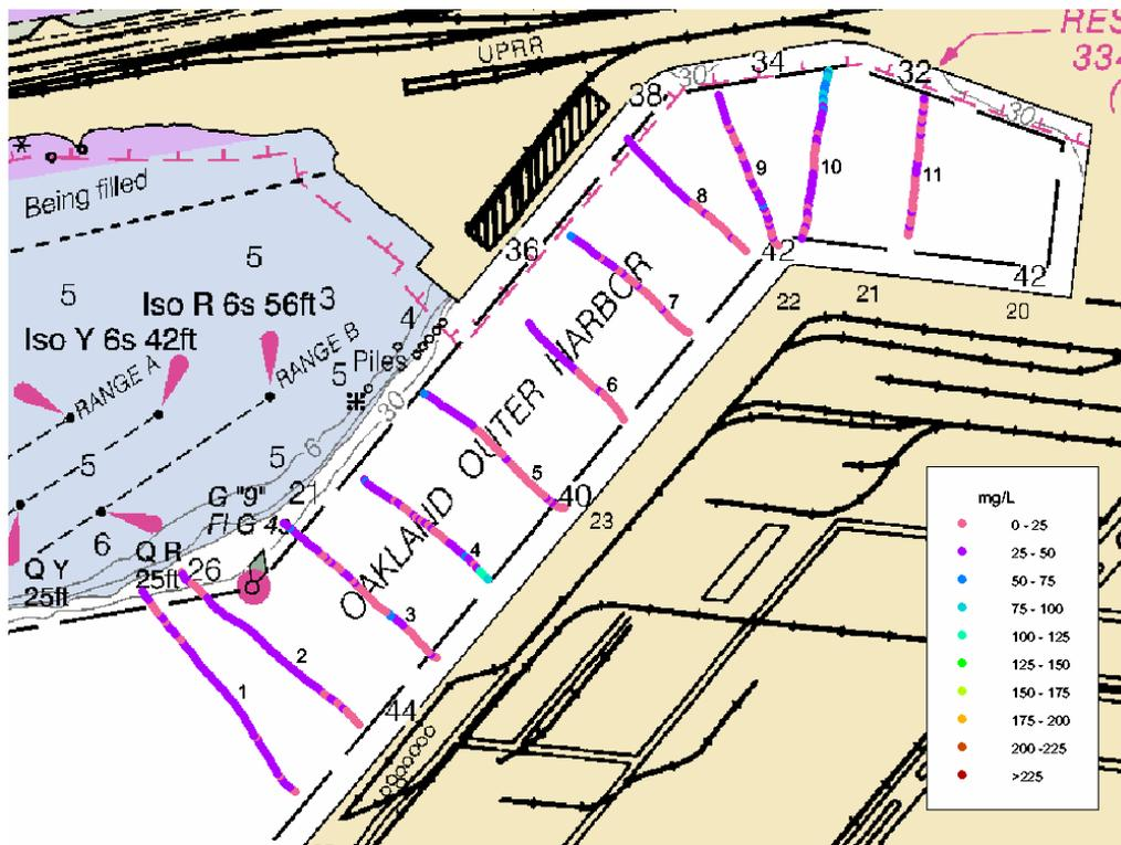
Figure 3. Depth-averaged acoustic estimates of suspended sediment concentrations during a period of dredging inactivity on an ebbing tide.
