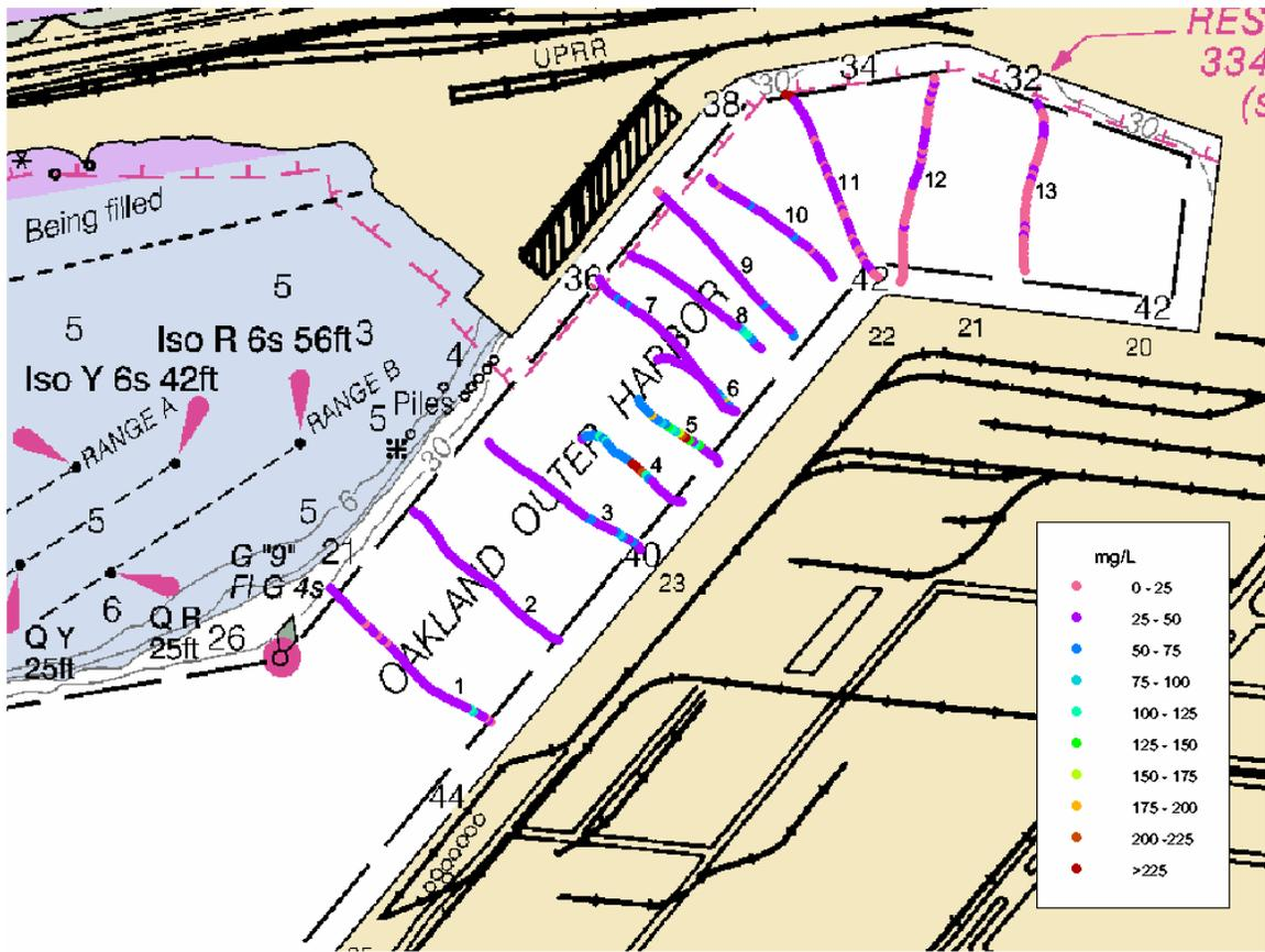
Figure 17. Locations of ADCP Survey ODFD transects during a flooding tide. The dredge was operating adjacent to Transects 4 and 5. Depth-averaged acoustic concentration estimates are indicated by color-coded dots.
