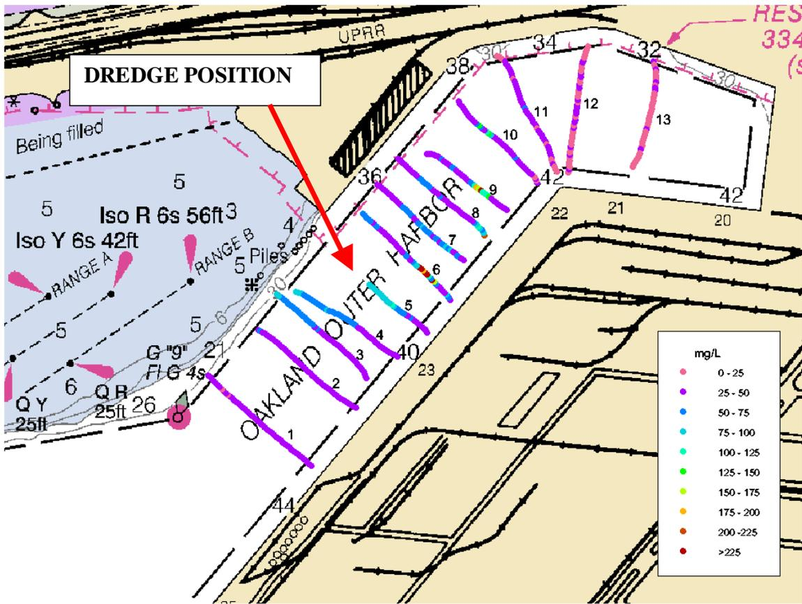
Figure 11. Locations of ADCP Survey ODFC transects during a flooding tide. The dredge was operating adjacent to Transect 5. Depth-averaged acoustic concentration estimates are indicated by color-coded dots.
