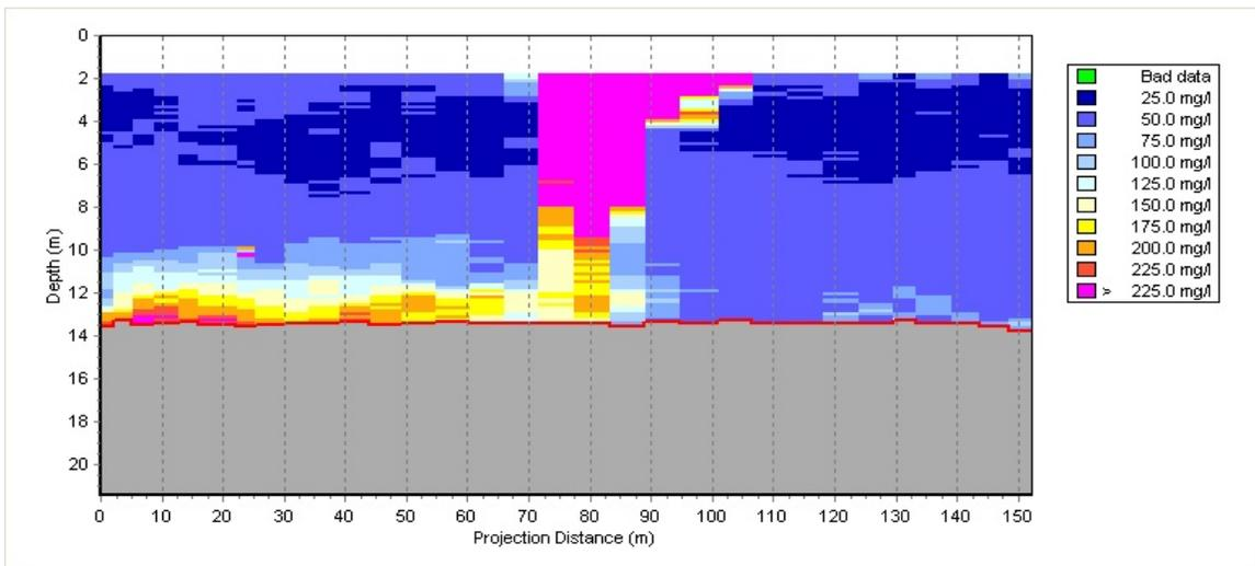
Figure 20. Vertical profile of TSS on Transect 4 during a flooding tide survey (ODFD).
