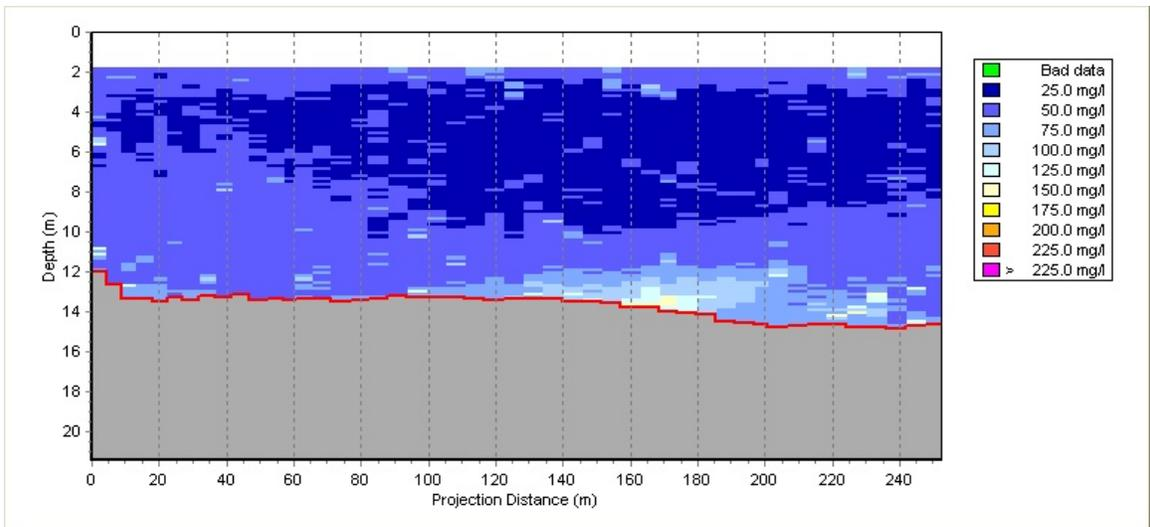
Figure 18. Vertical profile of TSS on Transect 2 during a flooding tide survey (ODFD) Harbor.
