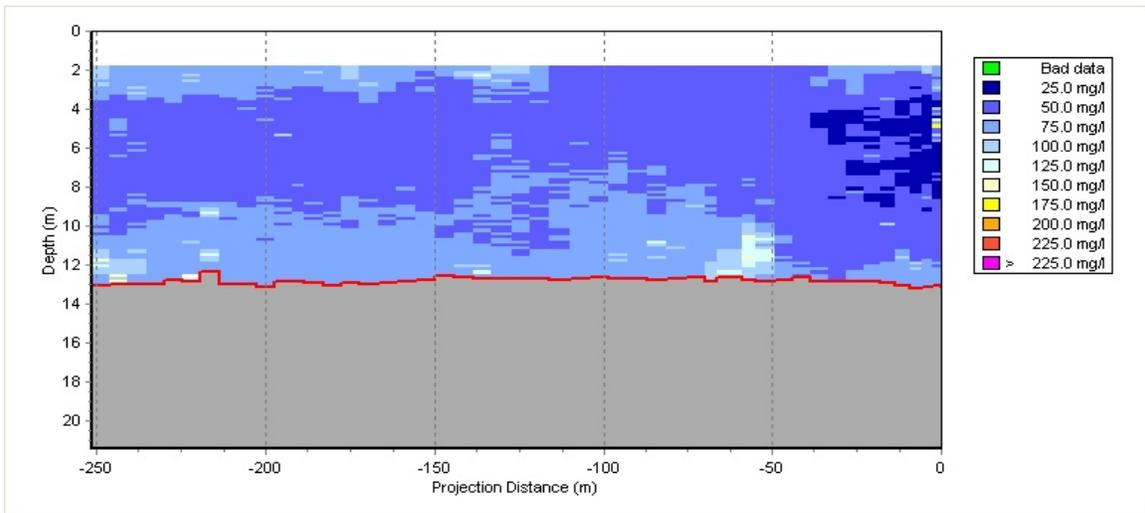
**Figure 14. Vertical profile of TSS on Transect 6 during a flooding tide survey (ODFC).**
