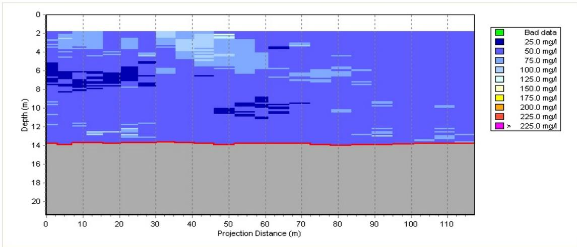
Figure 22. Vertical profile of TSS on Transect 6 during a flooding tide survey (ODFD).
