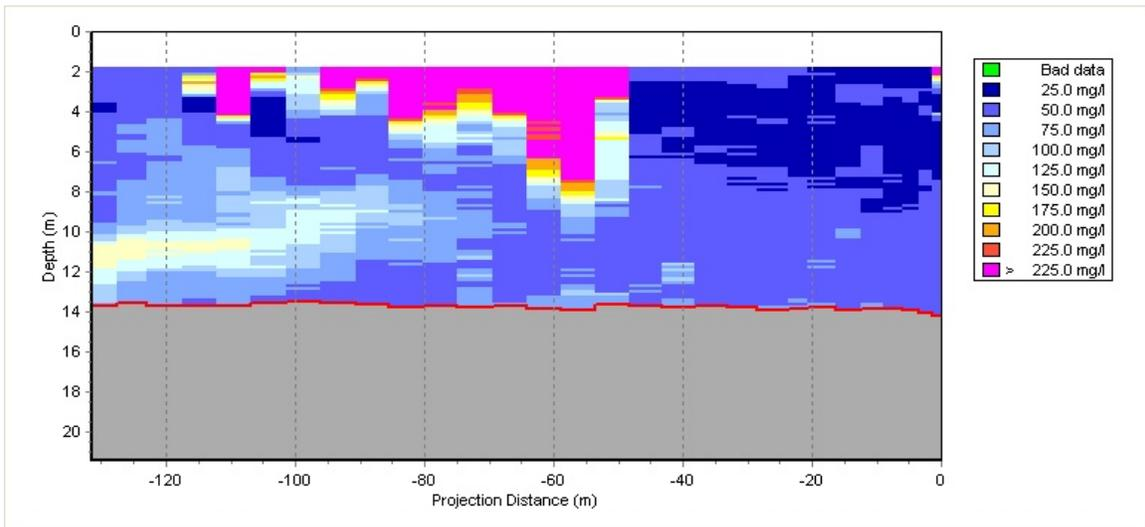
Figure 21. Vertical profile of TSS on Transect 5 during a flooding tide survey (ODFD).
