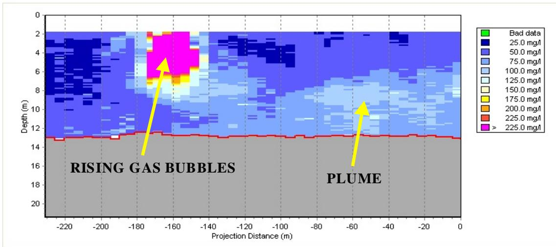
Figure 8. Vertical profile of TSS on Transect 6 during an ebbing tide survey (ODEC).
