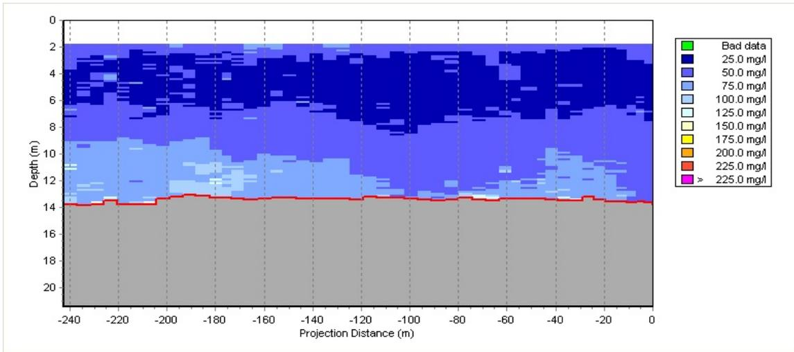
Figure 19. Vertical profile of TSS on Transect 3 during a flooding tide survey (ODFD).
