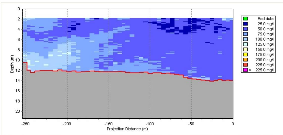
Figure 12. Vertical profile of TSS on Transect 3 during a flooding tide survey (ODFC).
