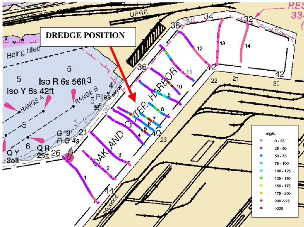
Figure 5. ADCP Survey ODEC transects during an ebbing tide. The dredge was operating adjacent to Transects 7 and 8. Depth-averaged acoustic concentration estimates are indicated by color-coded dots.
