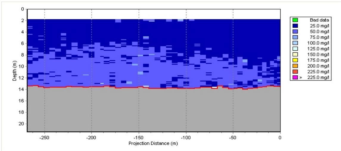
Figure 24. Vertical profile of TSS on Transect 12 during a flooding tide survey (ODFD).
