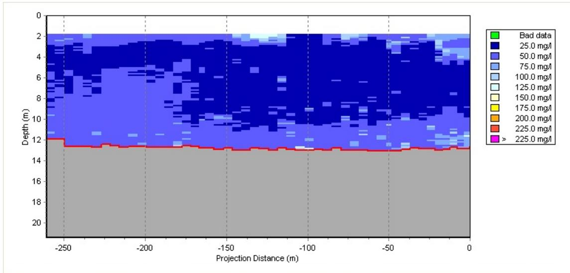
**Figure 10. Vertical profile of TSS on Transect 11 during an ebbing tide survey (ODEC).**
