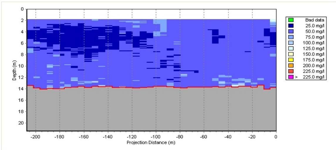
Figure 23. Vertical profile of TSS on Transect 8 during a flooding tide survey (ODFD).
