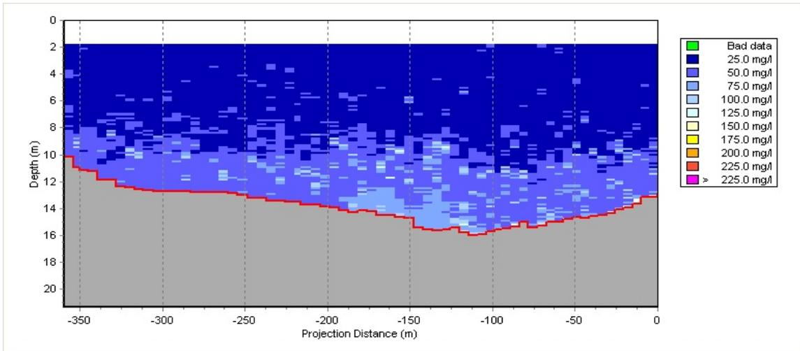
Figure 4. Vertical profile of ambient TSS on Transect 1 during an ebbing tide survey.
