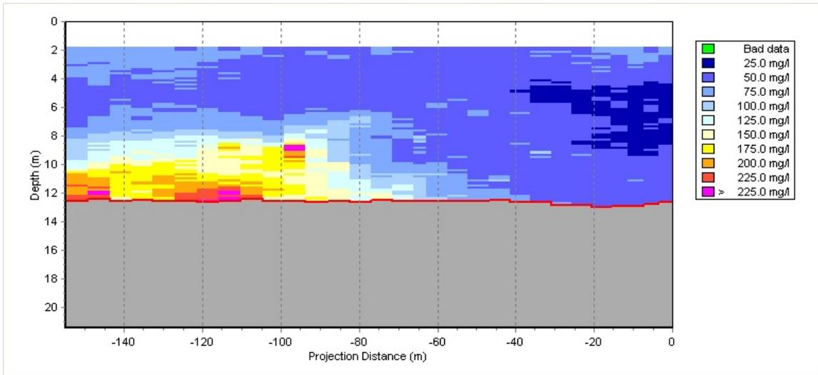
**Figure 13. Vertical profile of TSS on Transect 5 during a flooding tide survey (ODFC).**
