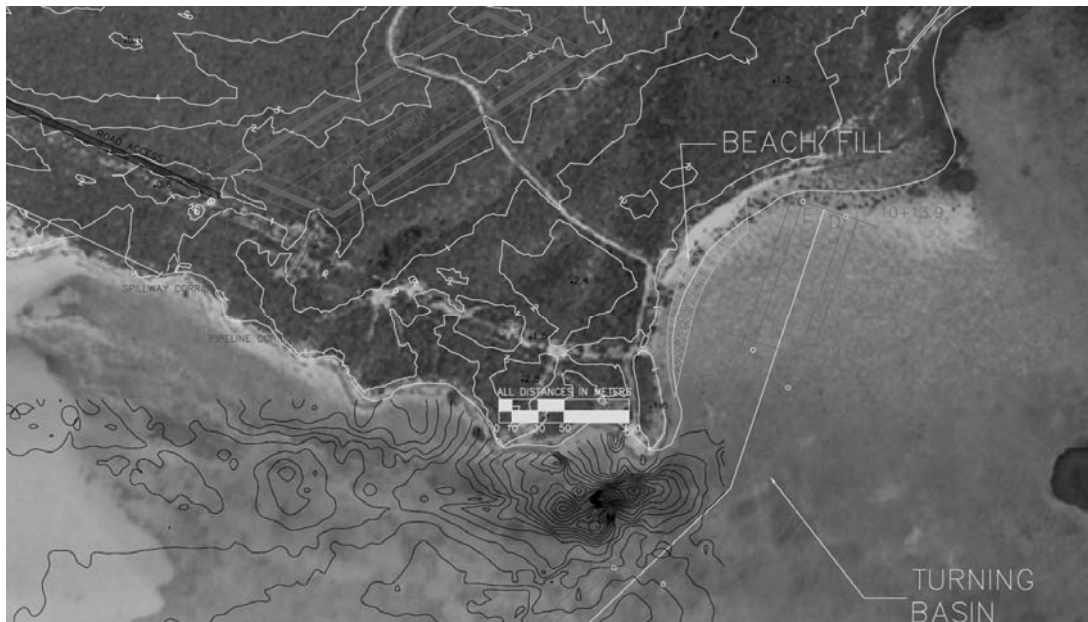
Figure 15. Water Cay Beach fill, Turning Basin, and Containment Area
