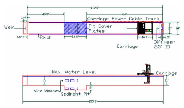
Figure 2. Plan and side view of the dredge/tow flume (dimensions in ft, divide by 3.28 for m).
