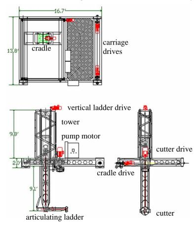
Figure 3. Dredge/tow carriage assembly drawing (dimensions in ft, divide by 3.28 for m).
