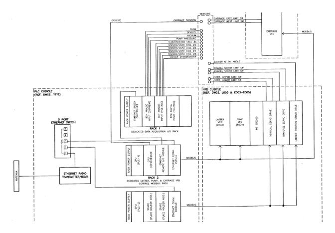
Figure 6. Electrical control and data channels for the dredge/tow carriage.
