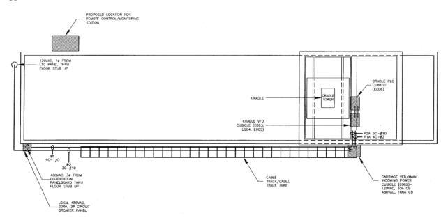
Figure 7. Electrical power cable track for dredge/tow carriage.
