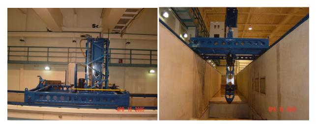
Figure 4. Dredge carriage sitting atop the dredge/tow flume (left) and the dredge ladder just above the sediment pit (right).
