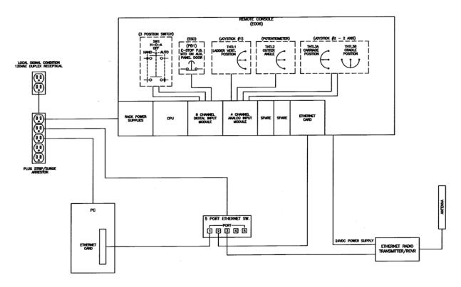
Figure 8. Schematic of SCADA and remote control console.
