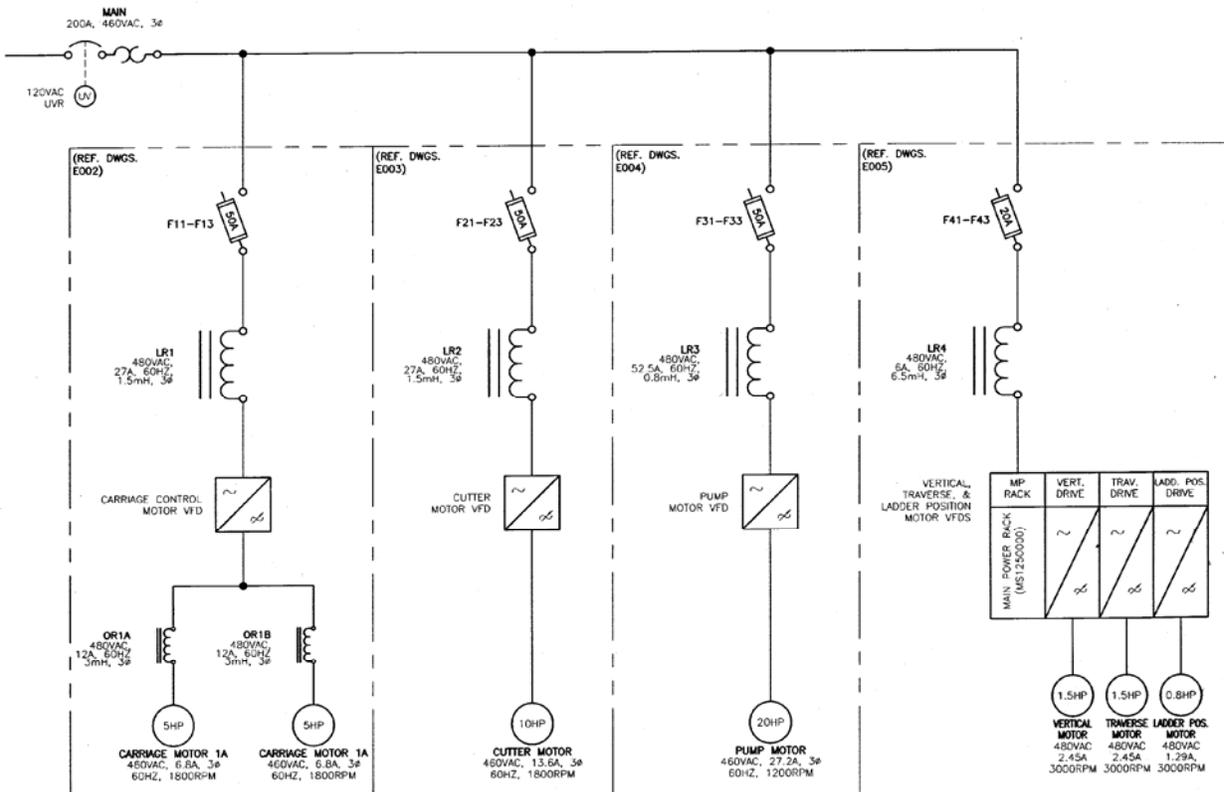
Figure 5. Electrical supply for dredge/tow carriage drive motors.
