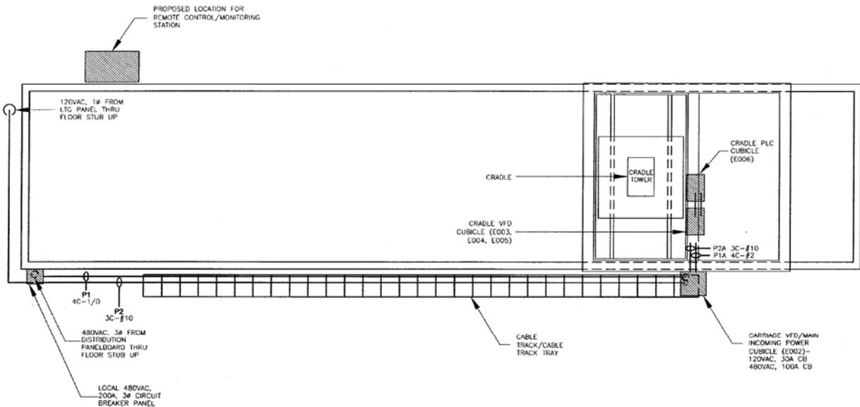
**Figure 7. Electrical power cable track for dredge/tow carriage.**
