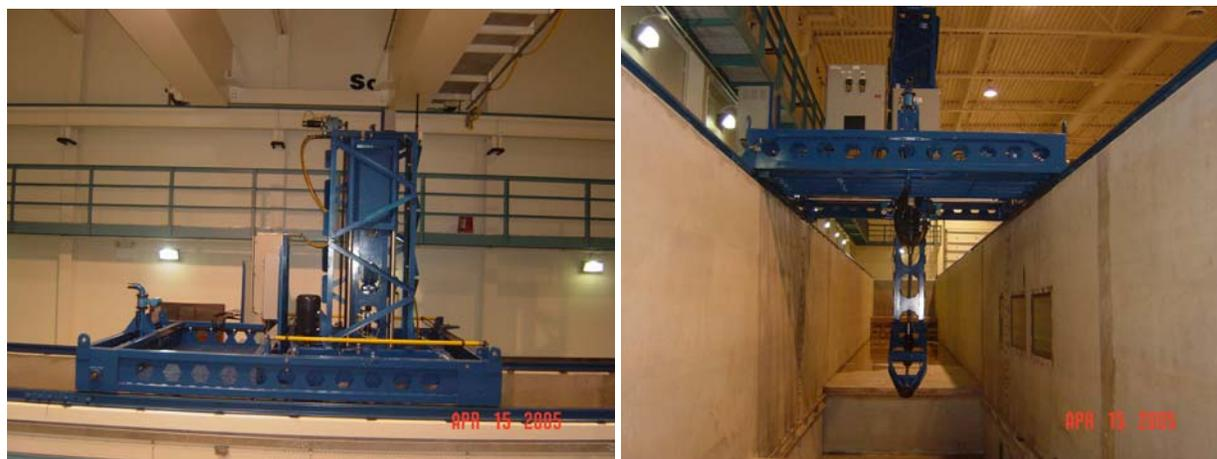
**Figure 4. Dredge carriage sitting atop the dredge/tow flume (left) and the dredge ladder just above the sediment pit (right).**
