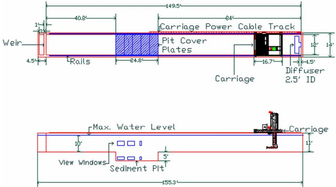
Figure 2. Plan and side view of the dredge/tow flume (dimensions in ft, divide by 3.28 for m).
