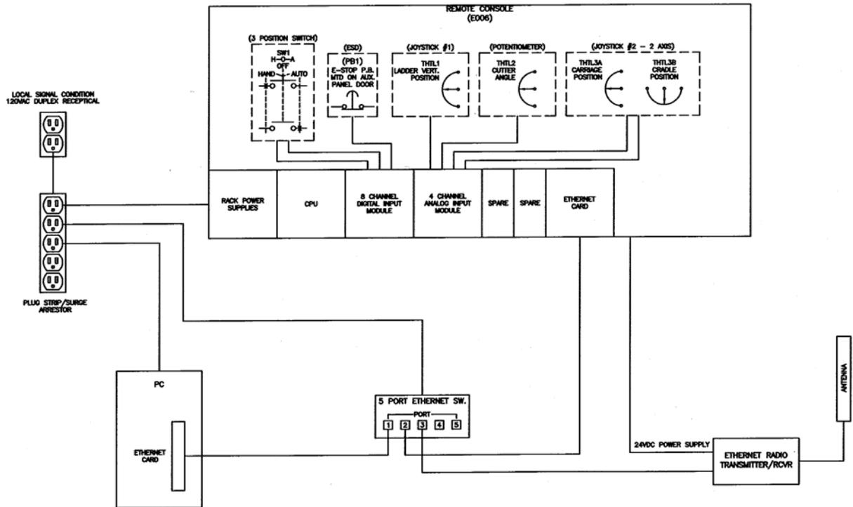
Figure 8. Schematic of SCADA and remote control console.
