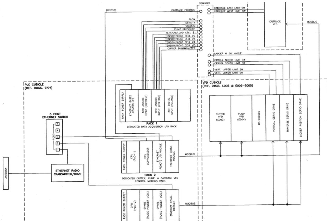
**Figure 6. Electrical control and data channels for the dredge/tow carriage.**
