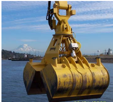
Figure 1. Young's closed hydraulic clamshell bucket for articulated fixed-arm dredge.
