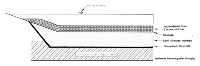
Figure 4. Cap schematic cross section.
