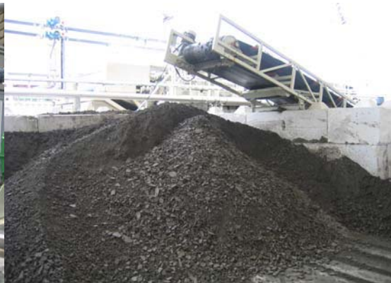
Figure 25. Sludge cake from belt filter press dewatering
