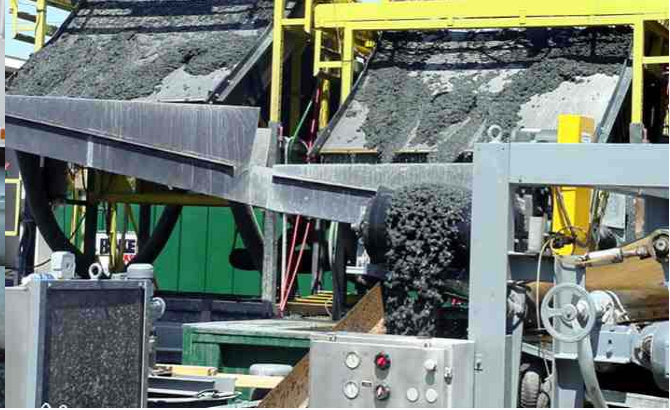
Figure 11. Thickened solids coming off the RDS® thickener
