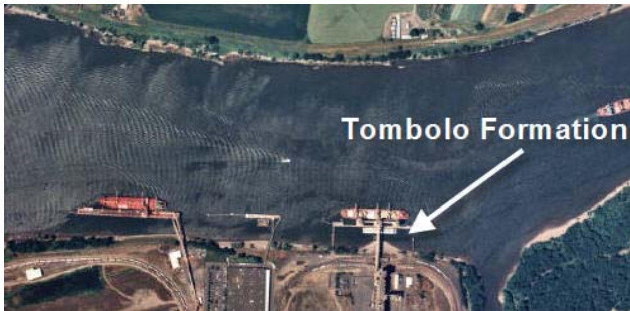
Figure 4. Typical tombolo at a grain elevator berth in Portland.
