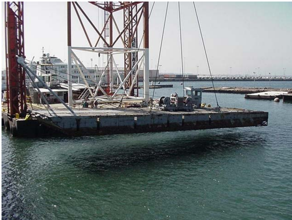
Figure 3. Warping tug lifted from water for transport from San Diego to Portland.
