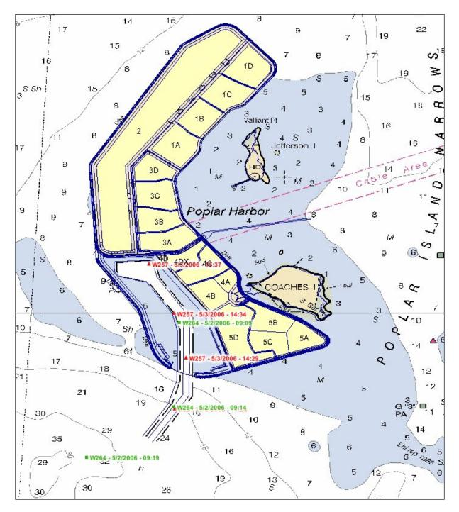
Figure 7. Online view of near real-time vessel positions for the 2005 Baltimore Harbor and Channels Maintenance Dredging illustrating the scows W257 entering the Poplar Island unloading facility and W264 departing.
