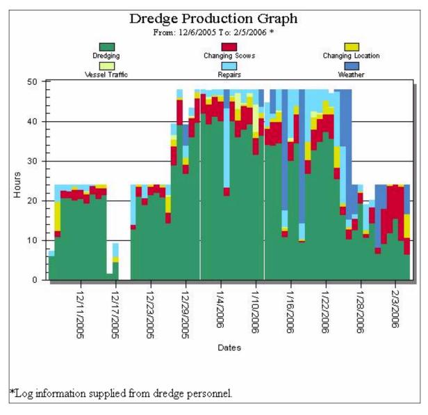
Figure 4. Online dredge production log data presented graphically for the dates 12/6/05 – 2/5/06 for one to two active dredges (24hr/days vs. 48hr/days).
