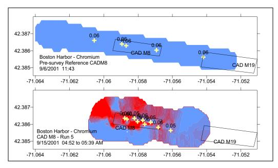
Figure 11. In situ turbidity values and chromium concentrations from discrete samples during background capping event surveys.
