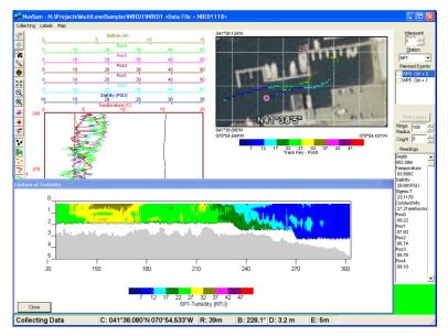
Figure 15. Real-time display during dredge monitoring survey.
