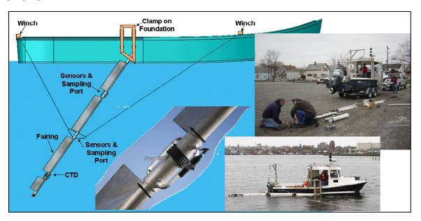
Figure 5. Views of the multi-depth water sampler.
