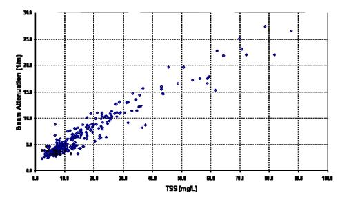
Figure 1. Results of calibrating transmissometer to measured total suspended solids.
