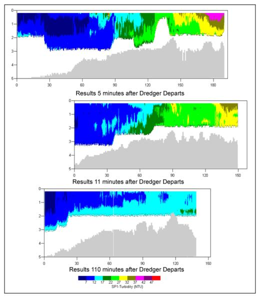
Figure 16. Three transects showing time-series of sediment plume evolution.
