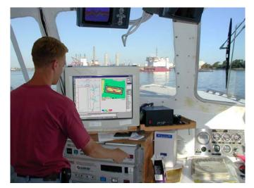
Figure 2. Real-time data acquisition system in use during capping operations.
