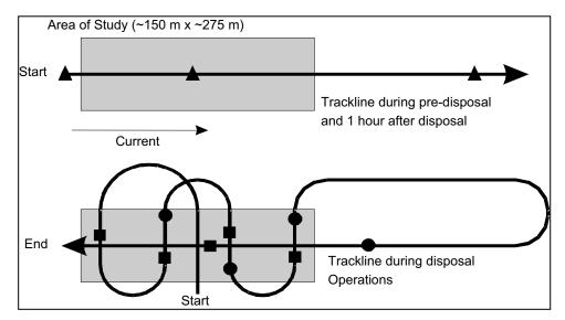
Figure 10. Preplanned survey tracklines and sampling locations.
