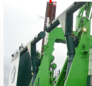
Barge Load Winch System
