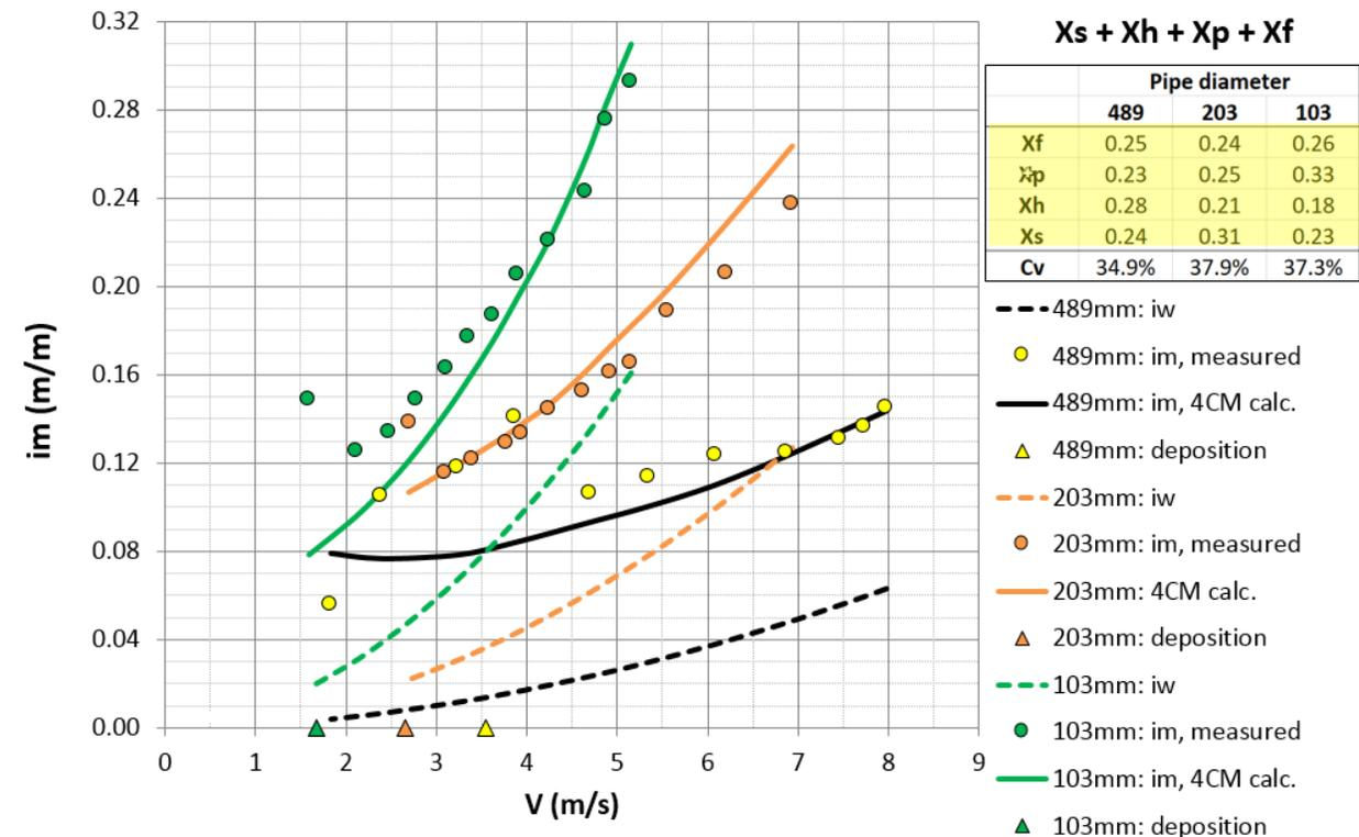
These figures show mixtures of three and four components respectively at volumetric concentrations near 35%. These tests represent concentrated slurries with broad particle size distributions. Note that the pressure gradients shown in these figures are comparable to the lower concentration, narrow PSD distributions seen in the previous slide.
