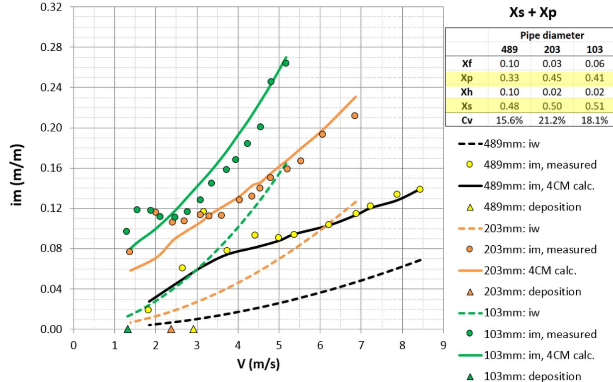
These figures show stratified  $X_s$  solids combined with heterogeneous  $X_h$  and pseudo-homogeneous  $X_p$  solids respectively.
