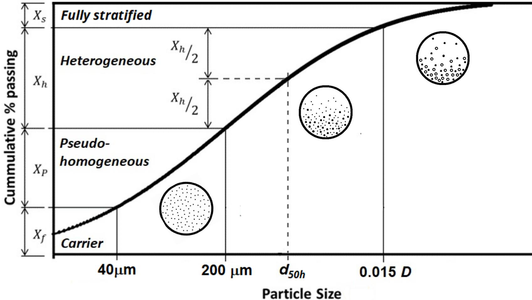
1. The slurry solids are divided into 4 groups or volume “fractions” based on the 4 basic flow regimes.
