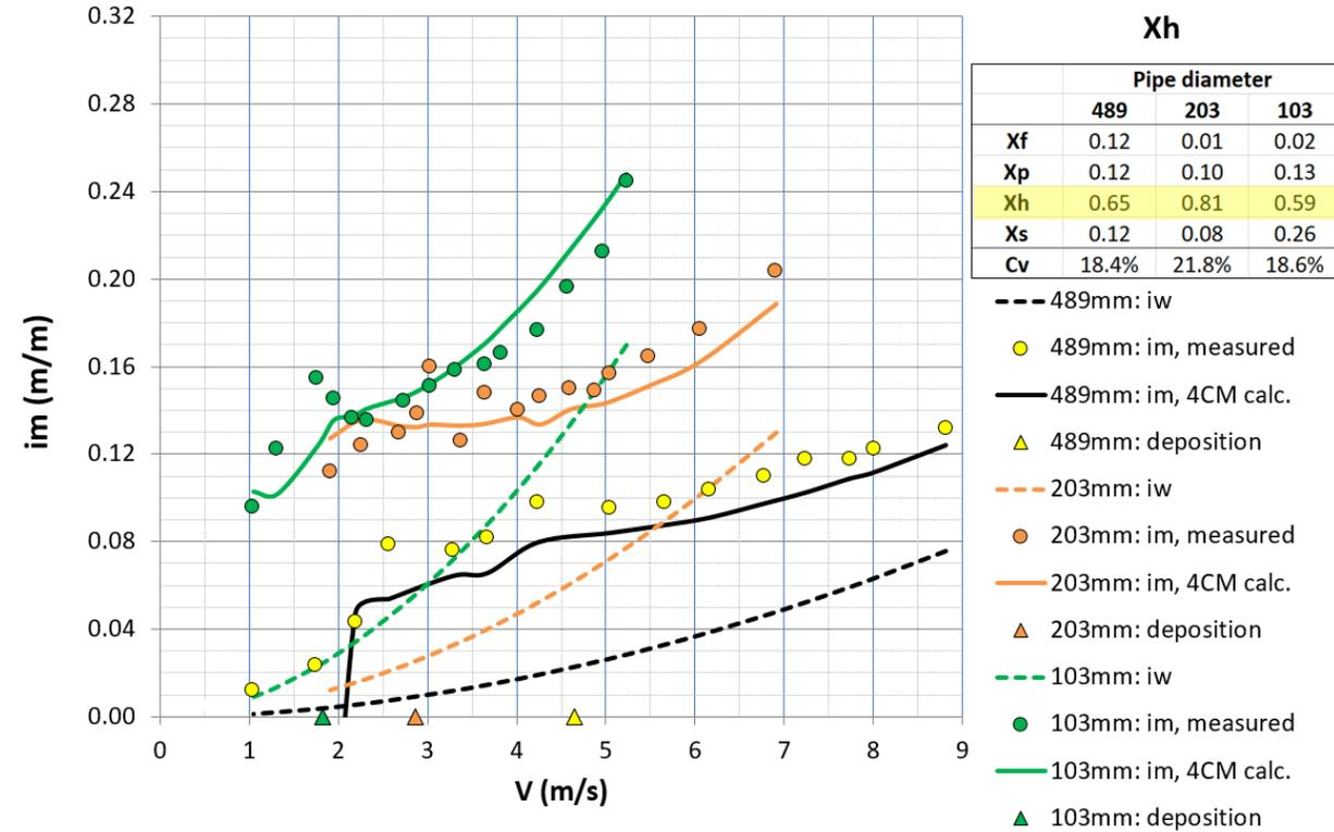
These figures show slurries where the single  $X_s$  or  $X_h$  components are dominant, resulting in relatively narrow particle size distributions. Volumetric concentrations are near 20%. Note the very visible effect of particle size and pipe size on the measured pressure gradient.
