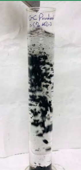
0.5% SedFirst-Treated Sand/5%PAC Uniform Distribution, No Dispersion
