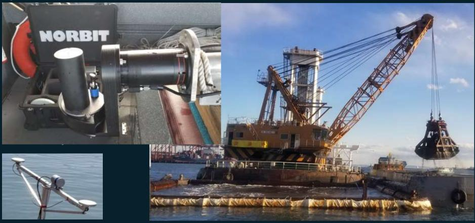
Dual head NORBIT **STX** with integrated **Lidar** and **GNSS/INS**
