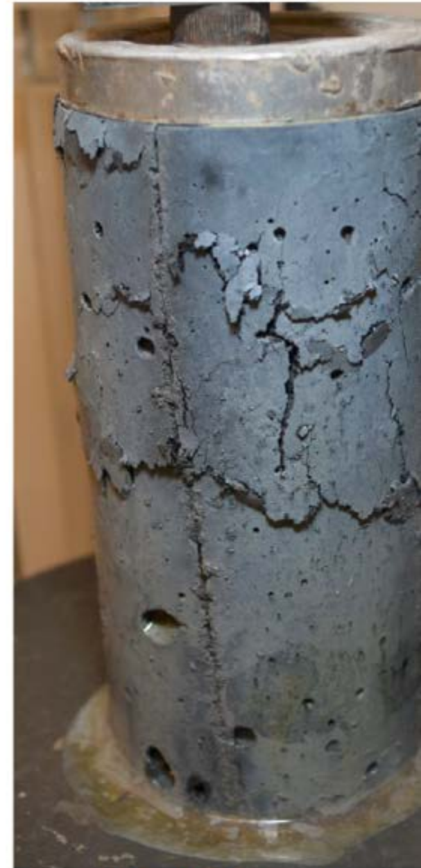
Failure Mode of Sample 4
