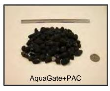
Sand/Gravel (100lb/CF Bulk Density) AG+PAC 10% (74lb/CF Bulk Density)
