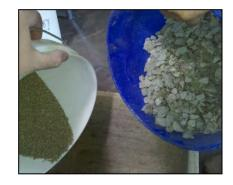
Sand/Gravel (100lb/CF Bulk Density) GAC (30lb/CF Bulk Density)
