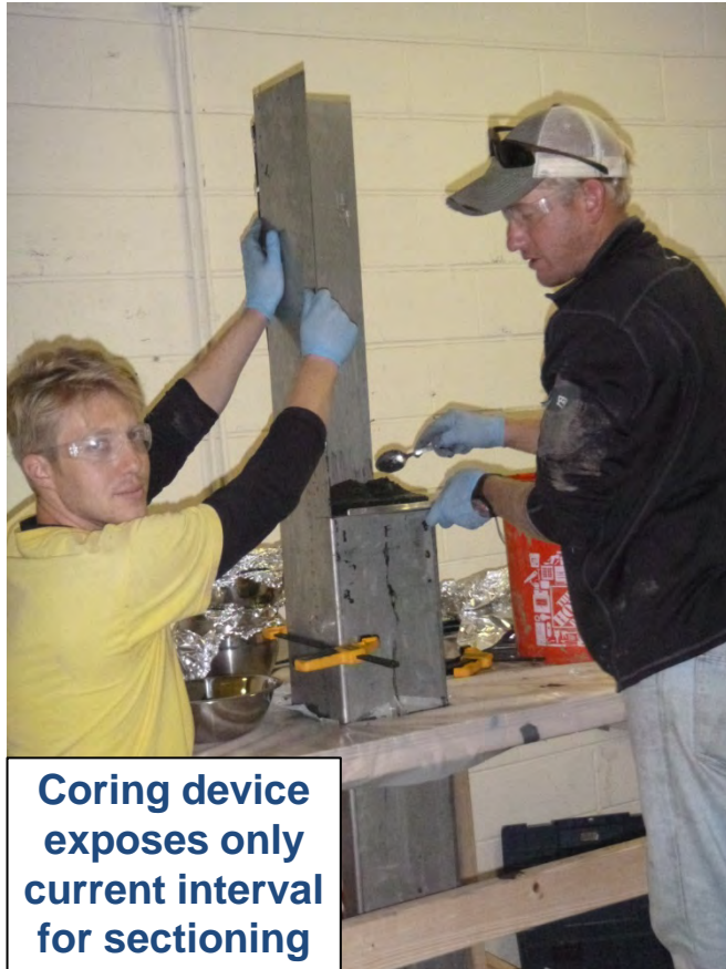
Stainless steel sectioning plates can cut through silt, sand, clay, and decayed organic detritus
