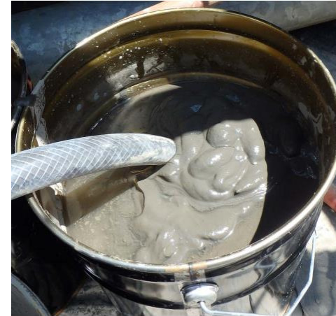
Clarifier Influent 1,500 gpm @ 3 – 12% d.s. (30,000 – 120,000 ppm TSS)
