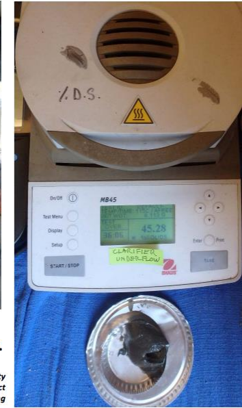
Clarifier/Thickener Underflow: 45% D.S.
