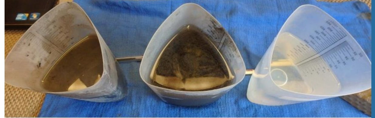
Clarifier Influent 1,500 gpm @ 3 – 12% d.s. (30,000 – 120,000 ppm TSS)
