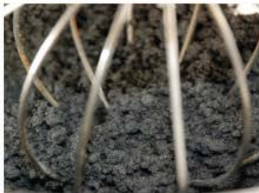
De-Agglomeration Phase Shearing of Large Bond Formations Exposing Residual Amendment To Latent Moistuer
