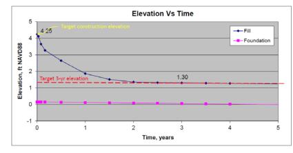
PSDDF - Primary Consolidation, Secondary Compression, And Desiccation Of Dredged Fill
